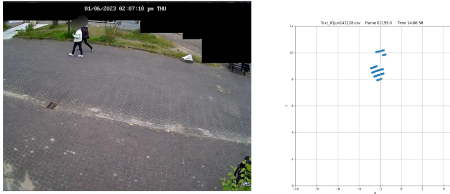
Figure 4.3: The radar output was marked into their respective classes using the Lassoselector Tool based on the camera data.
