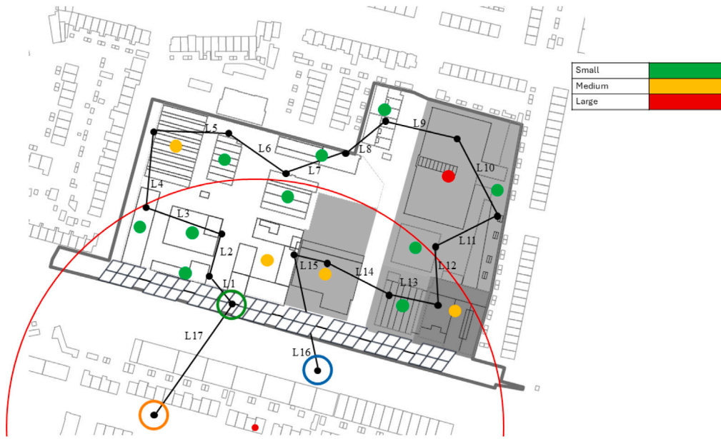
Fig. 5. Map of the heating network in Hilversum Werf, indicating the location of the centralised ATES.
