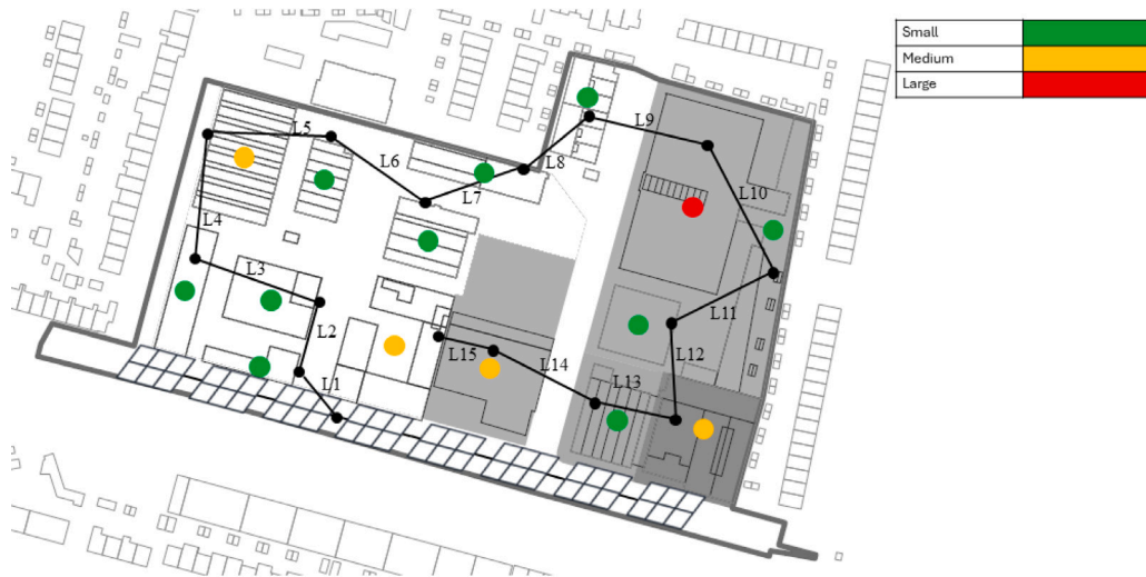
Fig. 1. Map of the heating network in Hilversum Werf, indicating the building categories.
