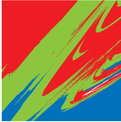
Figure 5.10: Basins of attraction for a seven-dimensional Double Gauss optimization problem. The initial curvature of the first surface is plotted vertically, and the initial curvature of the second surface is plotted horizontally.
