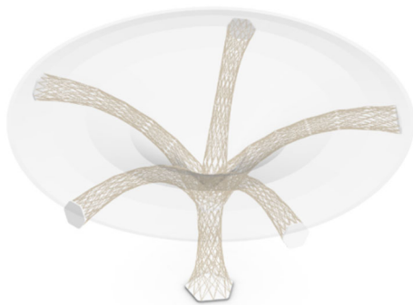
Figure 4: Fibrous tree column (Research-by-Design) Steinfort, R.T. (2024)
