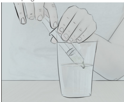
Press the syringe vacuum and pull to suck the silicone
