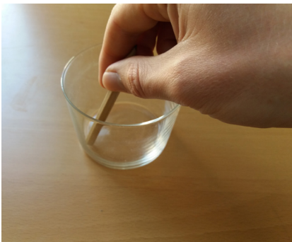
4. Mix the silicone components for 30 seconds with a stick.
