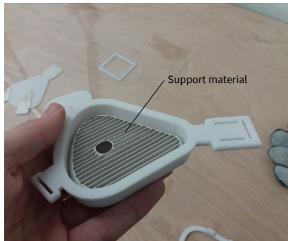
17. Remove the support material with a sharp pin after the 3D print is finished.
