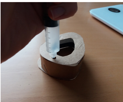
10. Inject the silicone into the casting hole, fully fill the mould.
