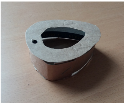
7. After the mould is finished, carefully lift it off the build platform and place it on a desk for the casting process.
