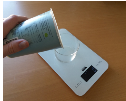
3. Pour the two silicone components of Ecoflex 00-35 in a cup (ratio 1:1) on a scale (at least 80ml in total).
