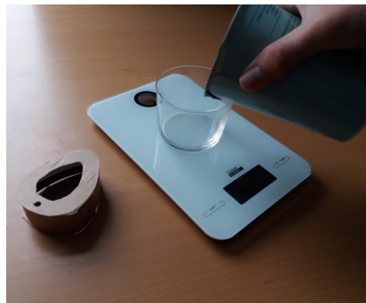
8. Pour the two silicone components of Dragon skin A20 (ratio 1:1) in a cup.
