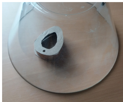
11. Place the mould in a vacuumed bell jar, to remove air via the gas vents.
