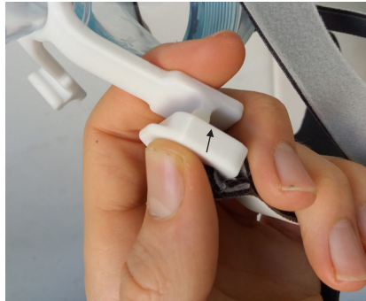
8. Place the mask onto the test participant's face, and fixate the mask by connecting the clips onto the holder.
