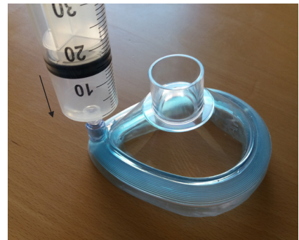
6. Screw the syringe on the inlet, and inject the cushion with 50ml of silicone.
