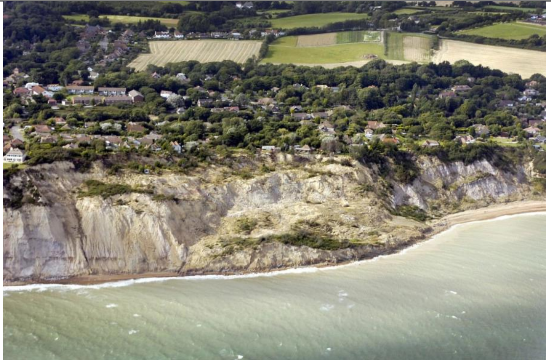
Figure 2: Effects on urban environment due to cliff instability caused by coastal erosion in Fairlight, East-Sussex, southeast England (Lycett, 2005).
