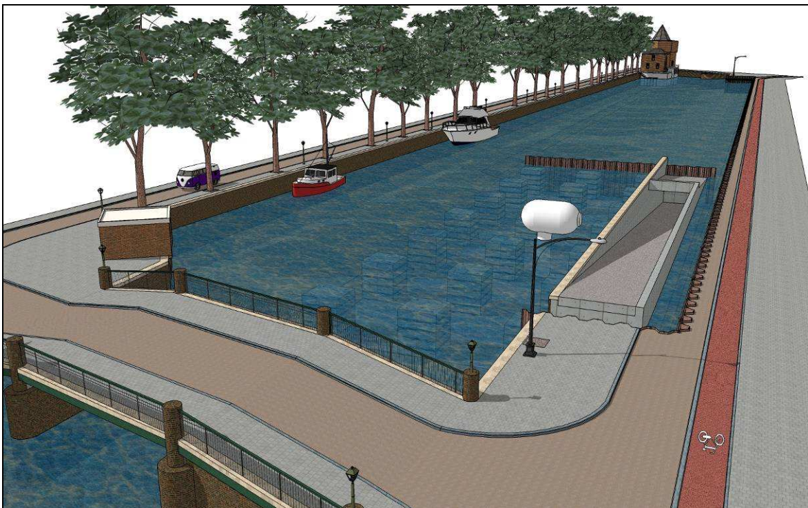
Figure I-9: Just before full immersion of the caisson, bricks and stones are placed applied on the new quaywall in dry conditions. After it is completely immersed, only the new quaywall, the ramps, the airlock and the sheetpiles rise above water.
