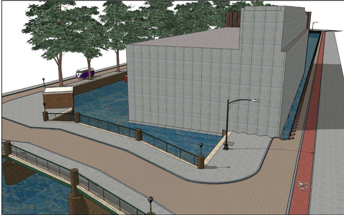
Figure I-6: If the caisson is not constructed and immersed in stages, the structure will rise up to +15m above street level. Besides the concrete works that shape the caisson, also some sheetpiles and locks are incorporated in the structure. These are needed in a later stage.
