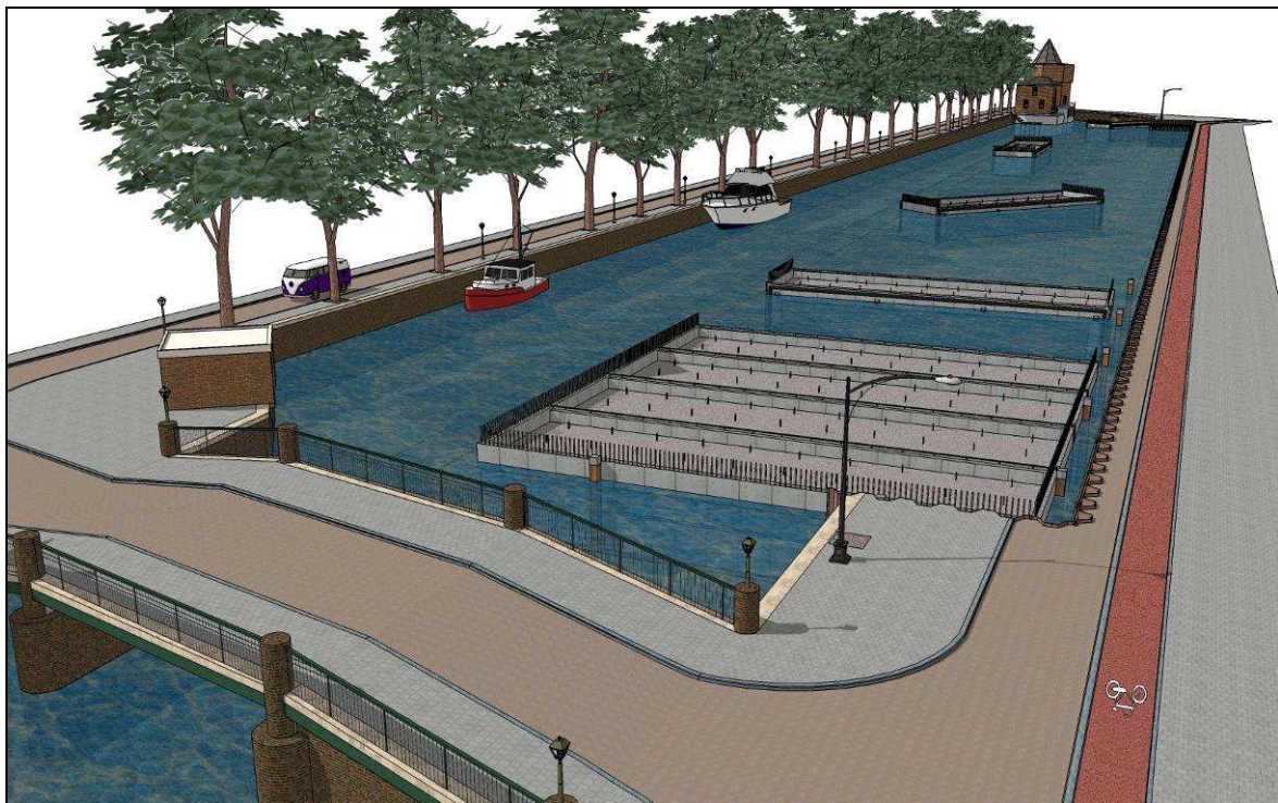
Figure I-3: The prefabricated elements are constructed off-site. After dredging of the canal, the elements are transported to the construction site over water. Once there, they are positioned and coupled with the aid of several spud piles.
