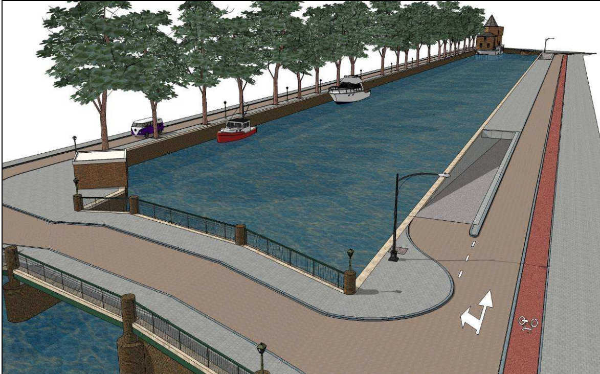
Figure I-13: A layer of sand is placed on top of the garage in the canal profile to protect it from damage. The space between the garage structure and the sheetpile walls is also filled up. After compacting of this sand, the sheetpile walls can be removed and pavement can be restored.
