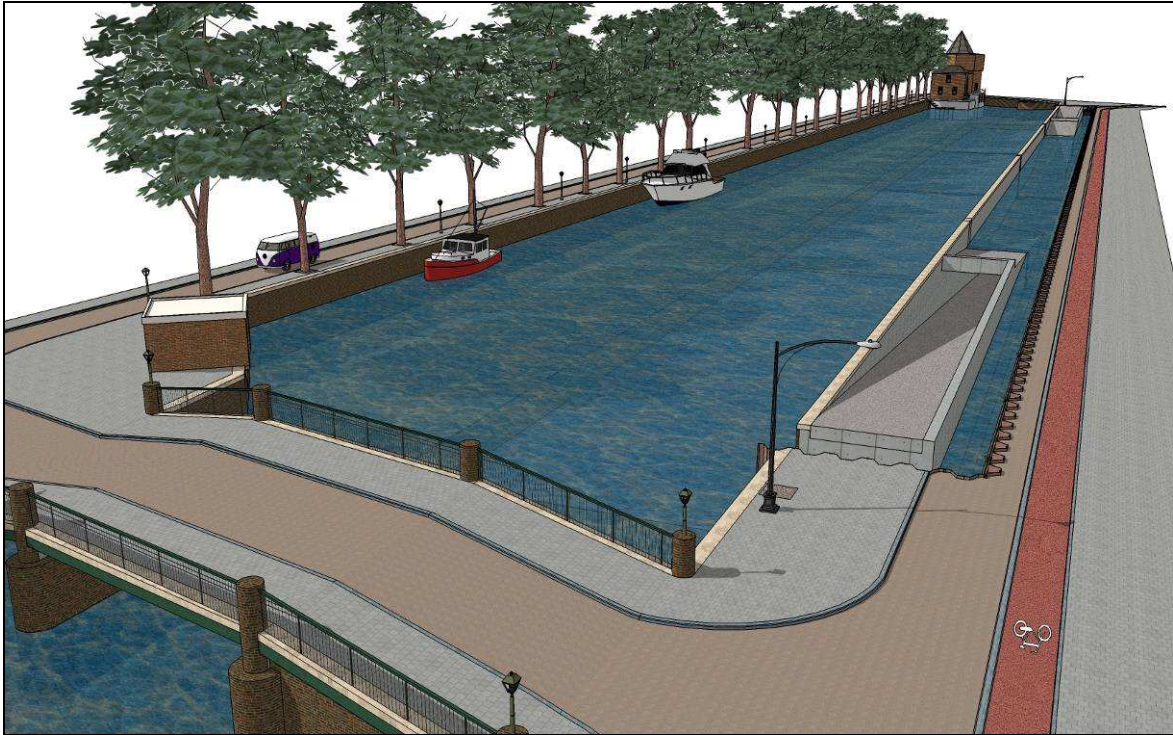
Figure I-12: As soon as the joints are made and the bulkheads are removed from within the caissons, the temporary retaining walls can also be removed. The carcass of the garage is now completed.
