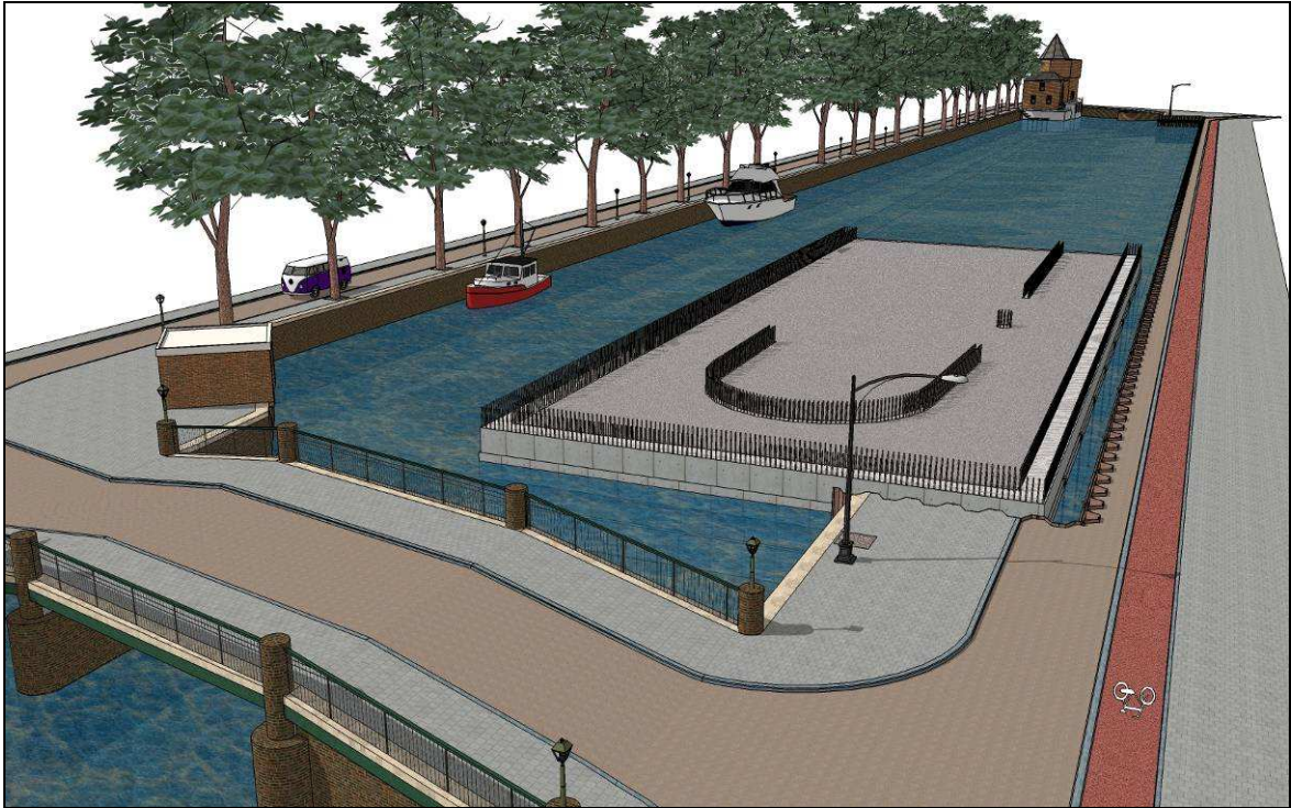
Figure I-4: When the prefabricated platform is fully assembled, it is immersed onto the canal bed and construction of the basement floor of the garage can commence on top of it.
