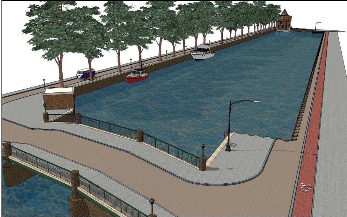
Figure I-2: After installing the sheetpile walls behind the eastern quaywall, trees are removed and the old quay is demolished. Traffic will temporarily be diverted several meters eastward, closer to the facades of adjacent buildings. (The tower at the far end of the canal represents the Schreierstoren.)
