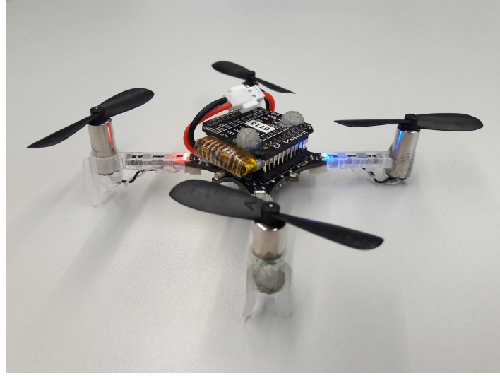
Figure 6-1: Crazyflie nano quadcopter used in this work. The gray reflective pellets are used for infrared tracking with the Vicon-system.
