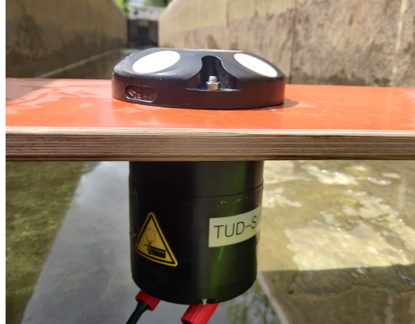
Figure 3.5: Testing of the bottom-mounted Signature1000 ADCP in a flume. Test measurements were conducted in multi-frequency mode at 1000, 500, and 250 kHz.
