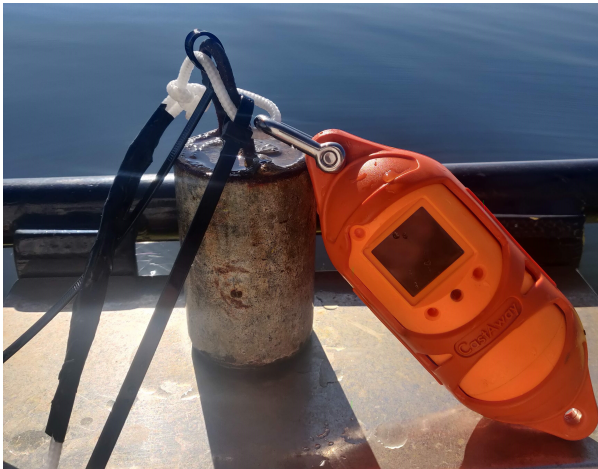
Figure 3.3: Sontek CastAway-CTD secured on a cable including extra weight.
