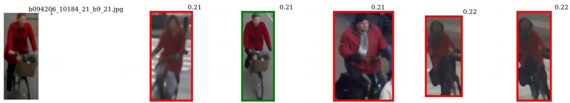
Figure 4.5: All of these images have a euclidean distance smaller than 0.6 and are classified as matches.
