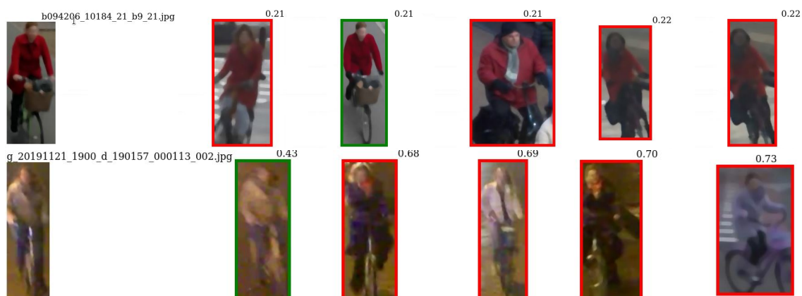
Figure 3.15: All of these images have a euclidean distance smaller than 0.6 and are classified as matches.
