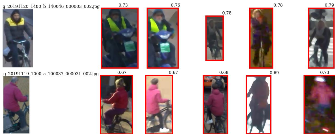
Figure 4.6: An example of re-identification from our blurred dataset, the green boxes contain the correct match while the red ones are mismatches. The distance mentioned above the images is the euclidean distance, the smaller the euclidean distance the more similar the images are. Here we see two distractors as input, and the returned euclidean distances are larger than 0.6 so these are correct.
