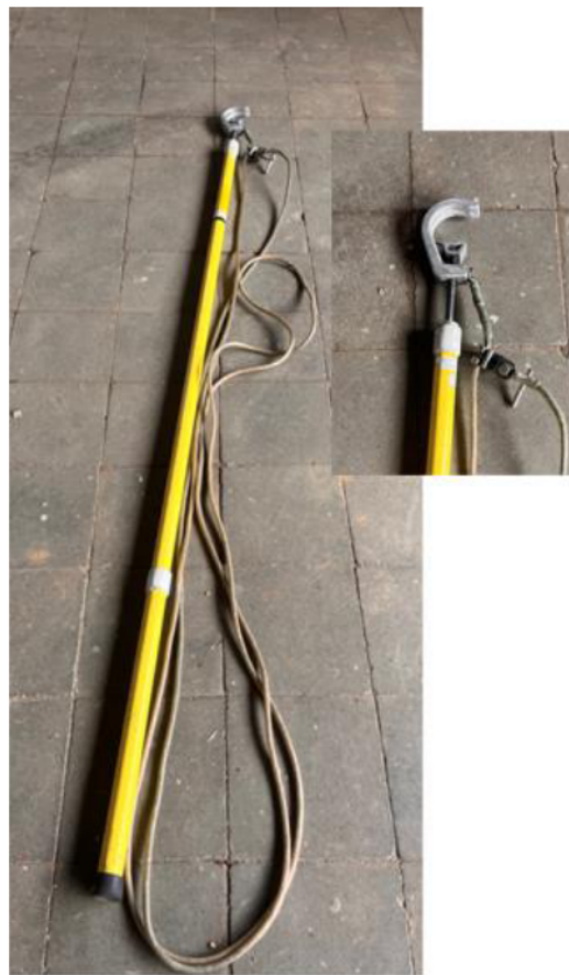
(b) Portable Earthing Device, from [1]
