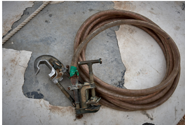
(a) Portable Earthing Device with Earthing Wire, from C.S. Engelbrecht
