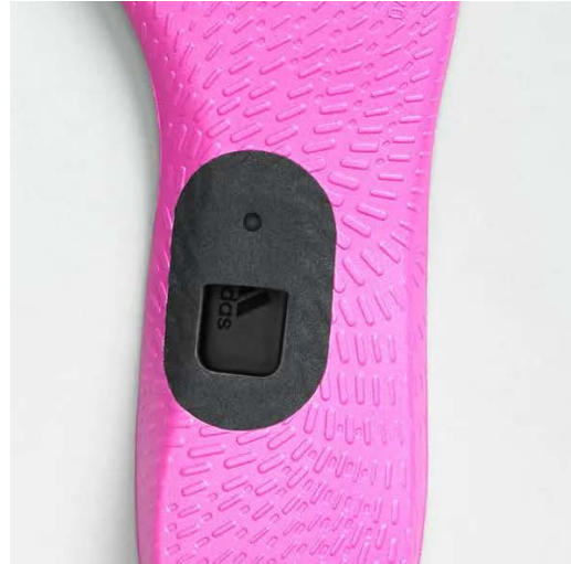
Figure 29: Jacquard module in shoe sole
