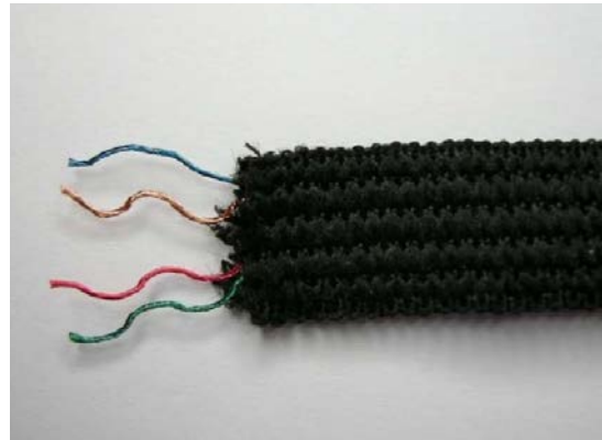
Figure 27: textile ribbon cable with embedded conductive wired
