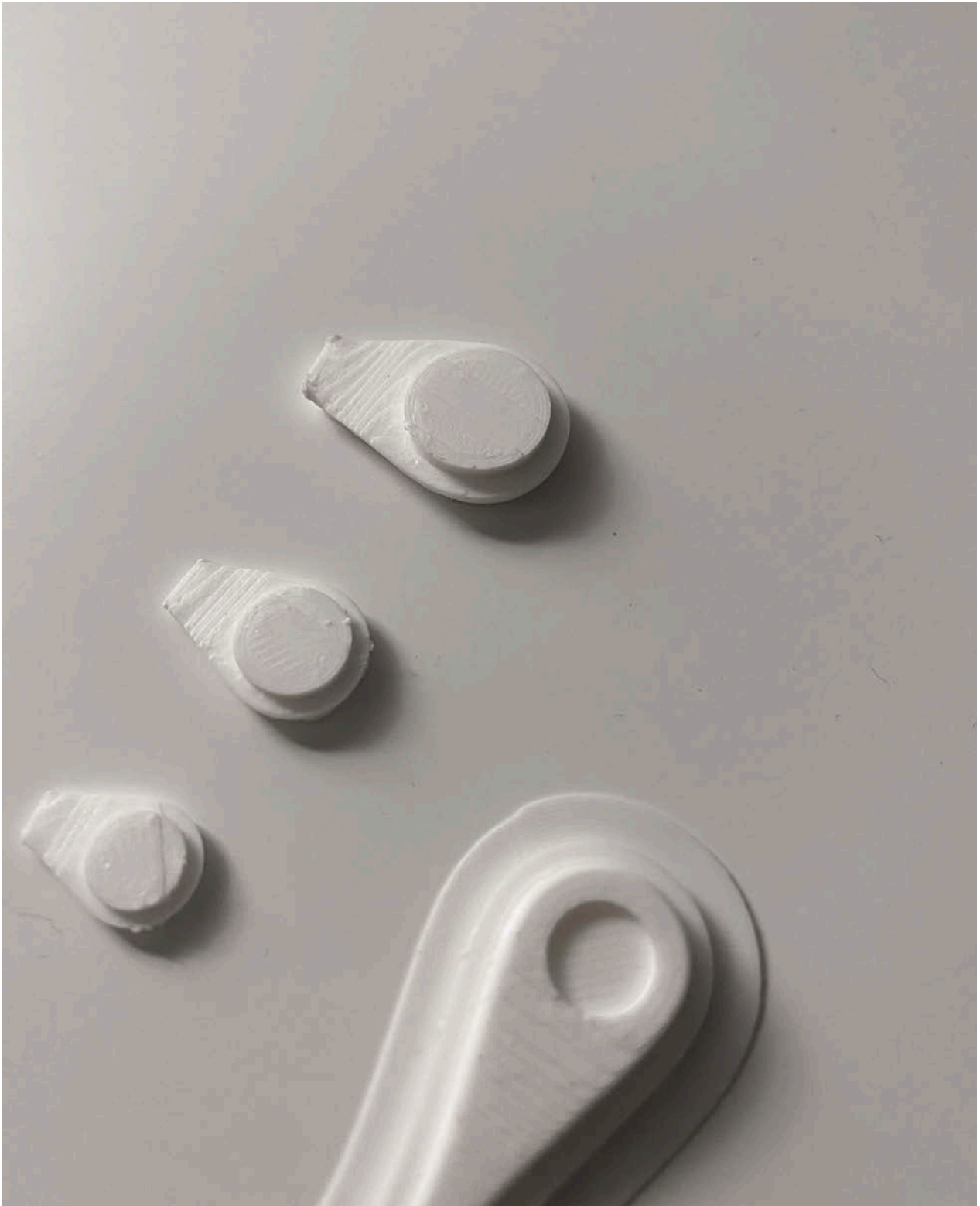
Figure 47: Three sizes for the connector that is to be places on the biosensor
