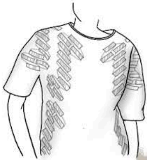
Earlier designs used T-shirts as carriers of the solar cells
