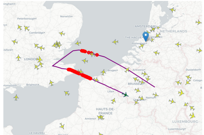
Figure 5. Estimated contrail formation based on the live trajectory data for one example trajectory.
