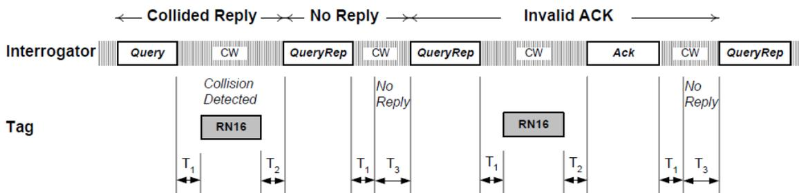
**Figure 2-21:** Procedure for collisions, empty slots and lost connections (source: EPC Global [3])
