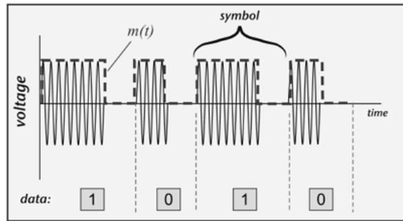
**Figure 2-16:** Pulse Interval Encoding combined with ASK (source:M. Dobkin [2])
