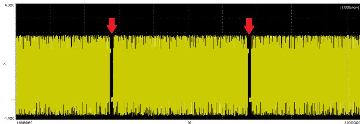
Figure 4-15: 100 Millisecond transmission break after at most 4 seconds of radiation
