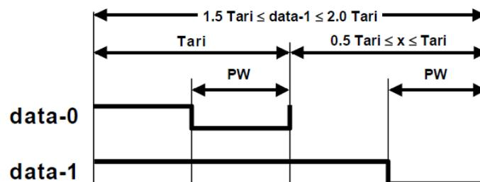
**Figure 2-17:** Pulse Interval Encoding (source: EPC Global [3])
