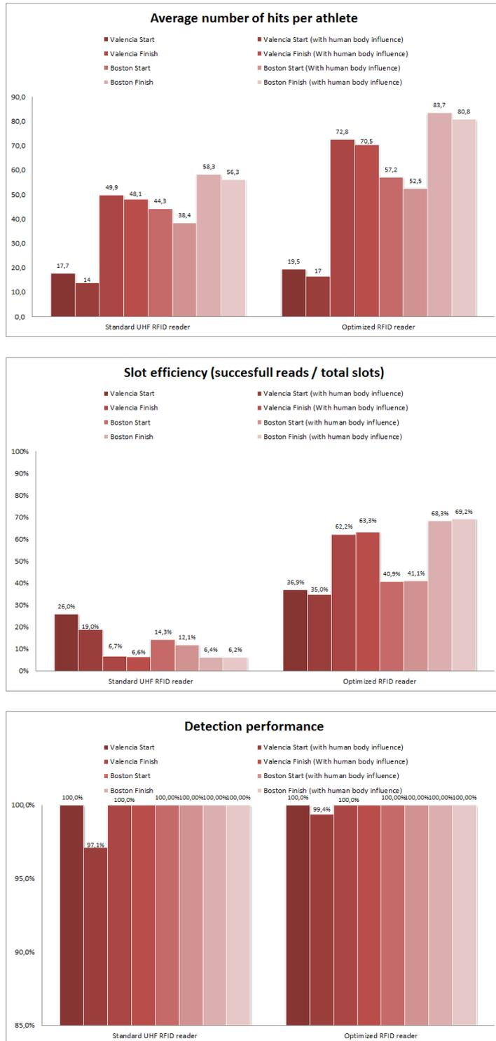
Figure 5-10: Simulation results: Standard UHF RFID reader vs Optimized reader
