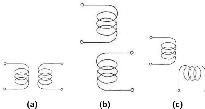
**Figure 2-12:** LF and HF tag orientation
