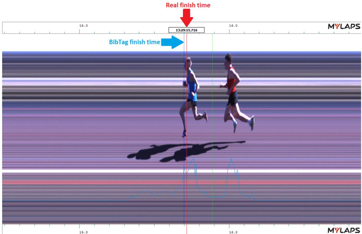
**Figure 4-10:** Example of test data recorded by the finish camera and BibTag system
