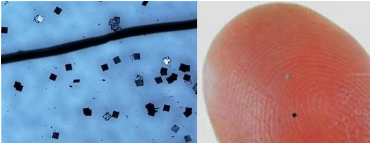
**Figure 2-2:** The smallest tag, 0.05 × 0.05 mm, compared with a human hair. (source:Hitachi)
