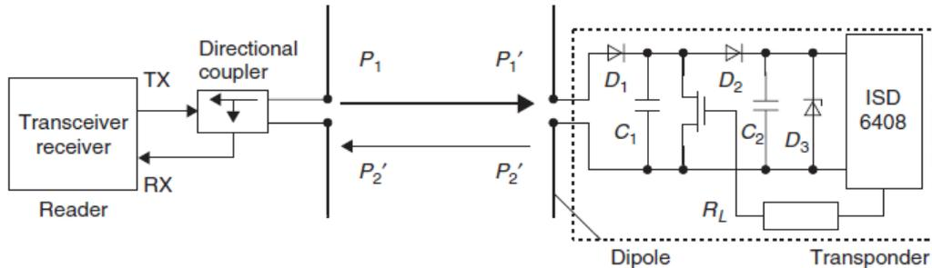
**Figure 2-6:** Backscatter for UHF and Microwave (source:Finkenzeller [1])
