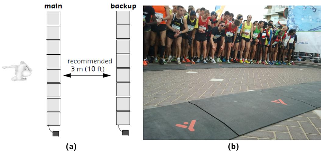
**Figure 4-12:** Two timing lines at the start and finish to reduce the probability of missing an athlete (source: MYLAPS)
