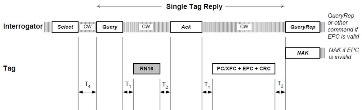
**Figure 2-20:** Single tag reading procedure (source: EPC Global [3])
