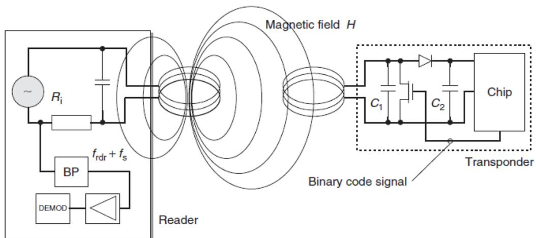
**Figure 2-5:** Inductive coupling for LF and HF (source:Finkenzeller [1])
