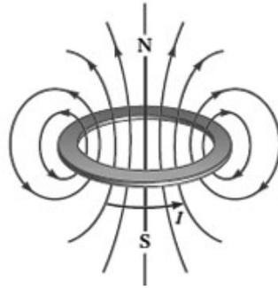
**Figure 2-11:** Magnetic field of a flat coil (loop antenna) (source: h2physics.org)
