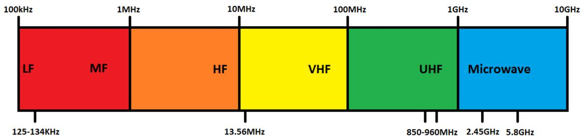
Figure 2-3: RFID frequency spectrum
