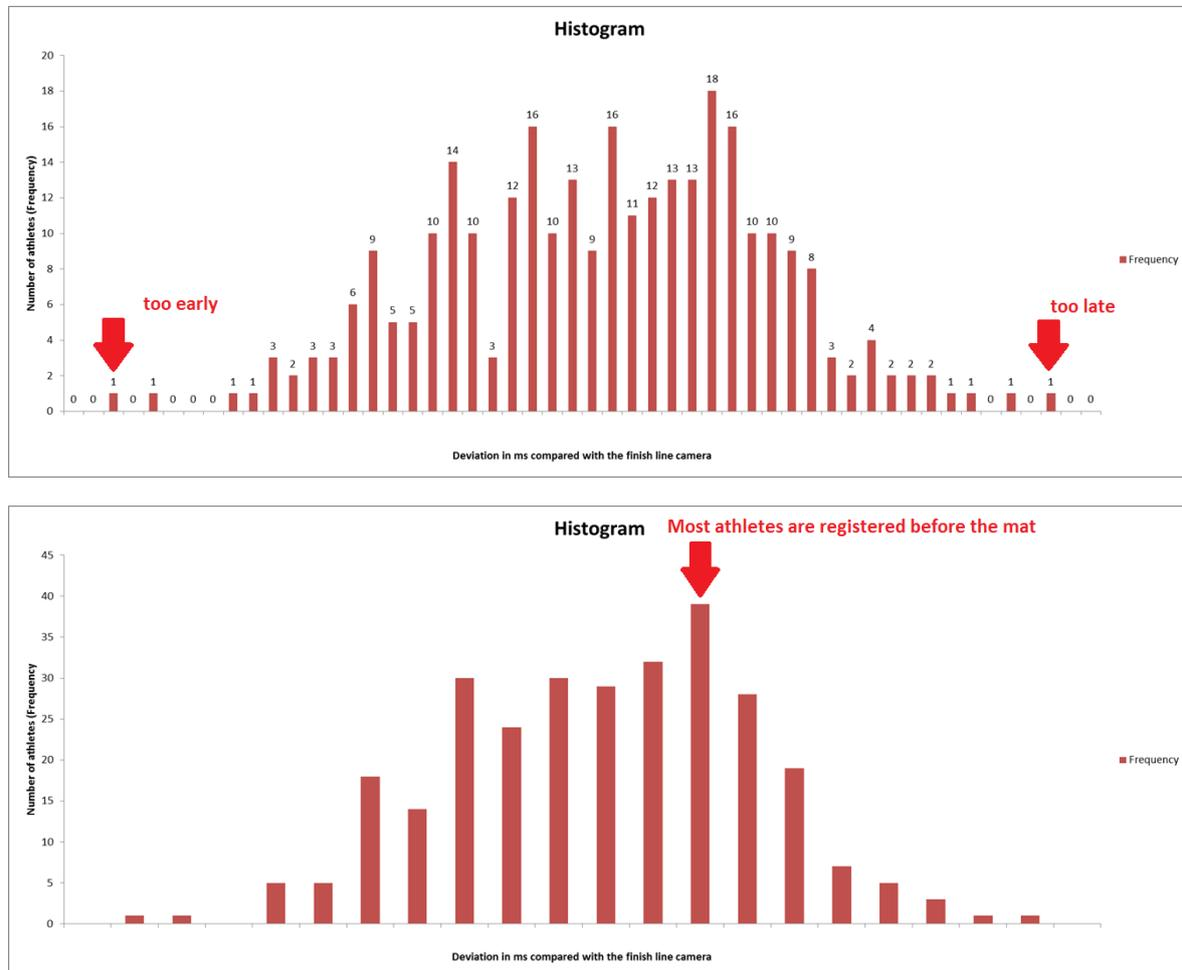
**Figure 4-11:** Time difference between the BibTag system and the actual finish time
