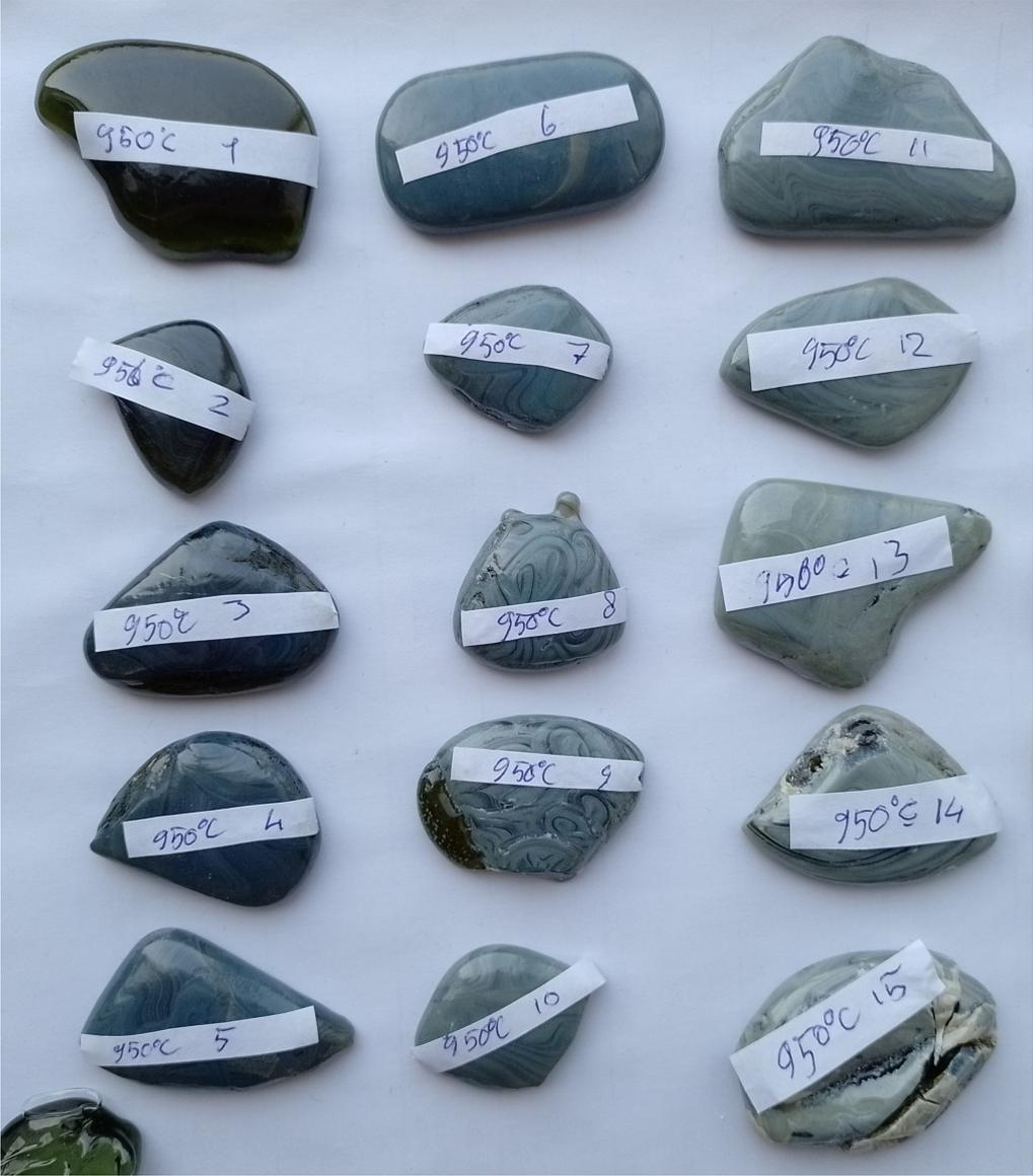
Figure 4.2: The samples which have been subjected to 950 °C for differing durations.
