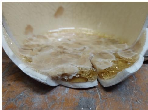
(a) The alumina crucible with a partially crystallized layer of glass melt.
