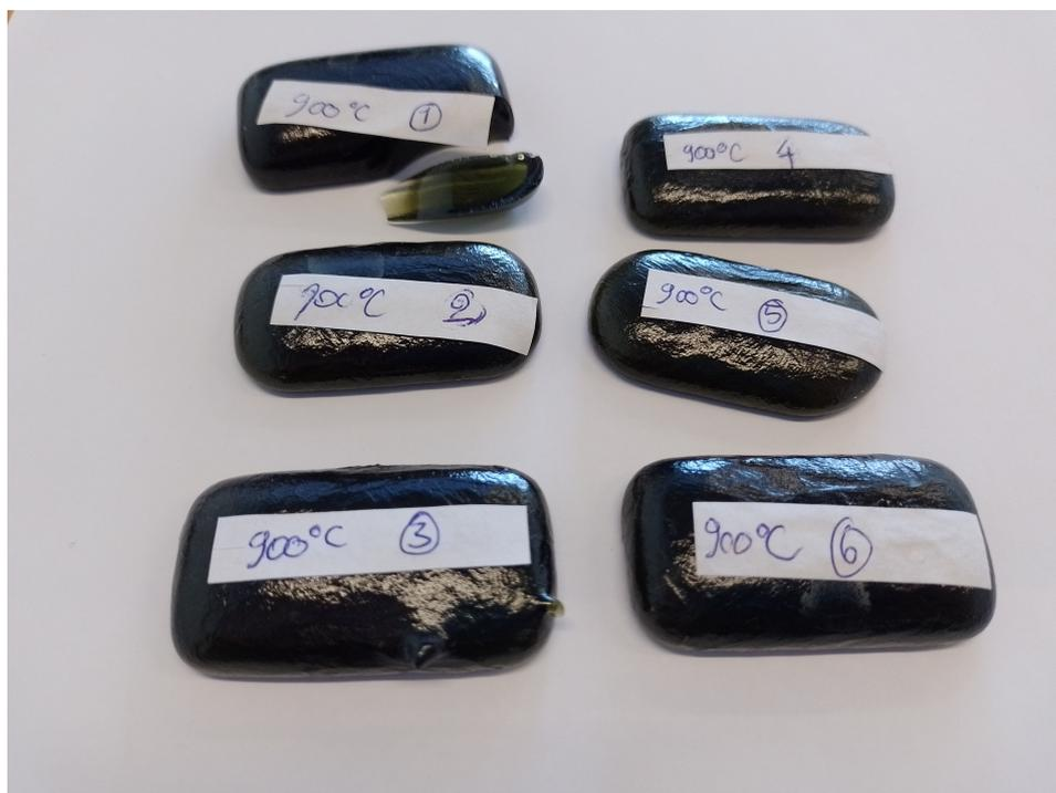
**Figure 4.1:** Six samples which have been subjected to 900 °C for differing durations
