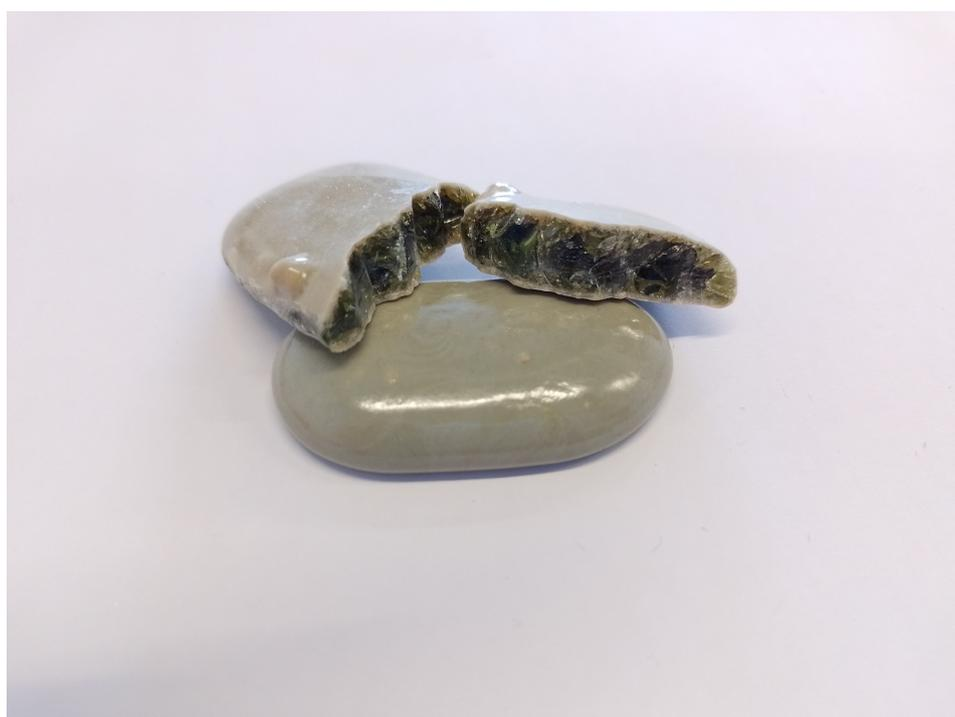
**Figure 4.3:** Some of the samples which have been subjected to 1000 °C for differing durations. One of the samples has split open and it can be seen that only the outer shell has fully crystallized, while the core remains glass.
