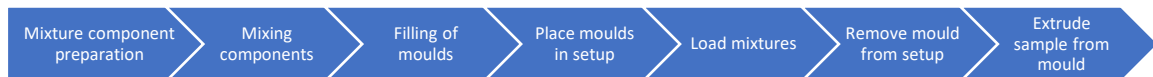
Figure D.2; Flowchart showing the process of the laboratory soil stabilisation procedure.
