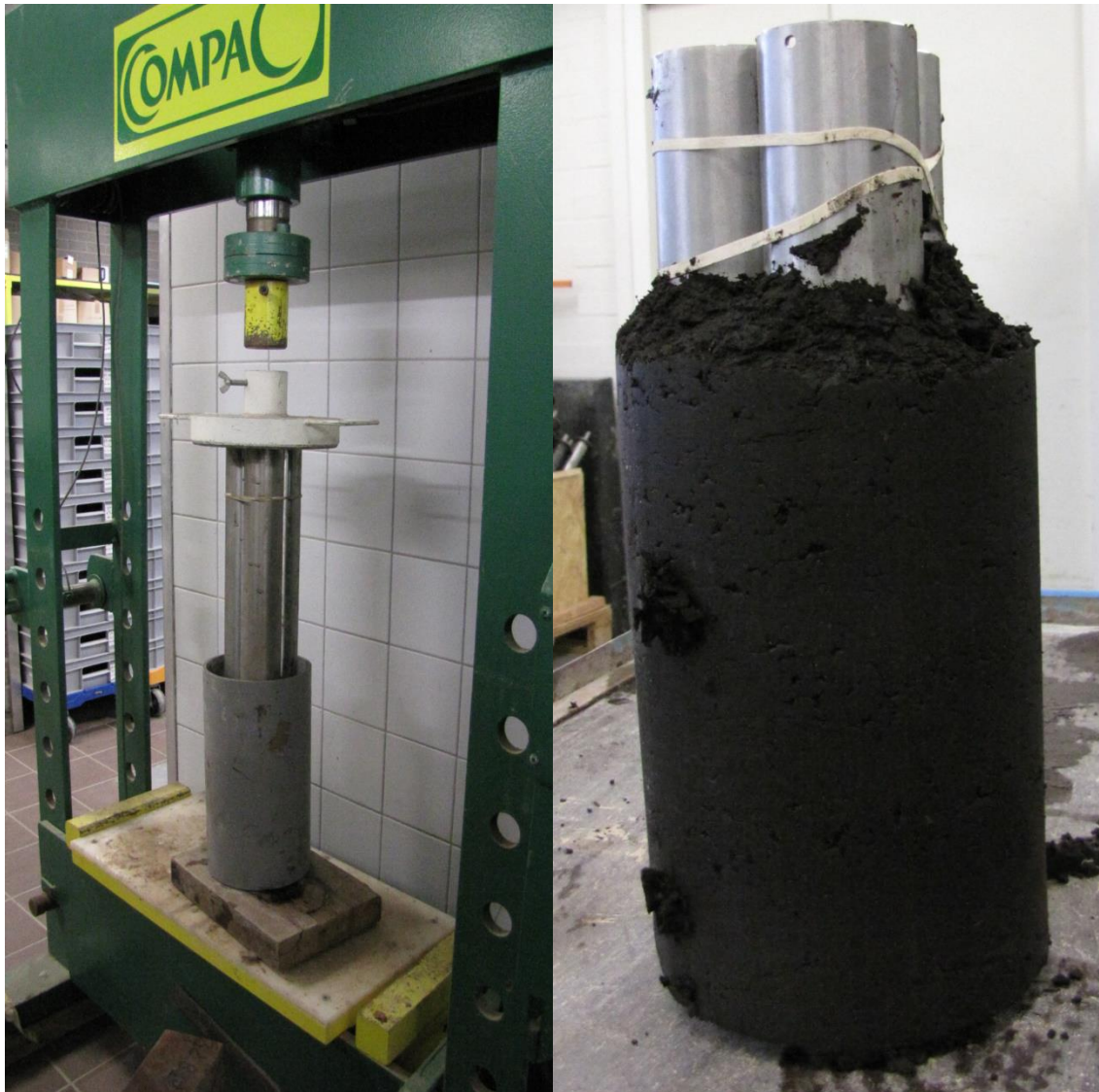
Figure D.10; The pushing of three small 50 mm diameter tubes into the stabilised soil sample in the mould using a compression machine (left) and the resulted extruded sample with the smaller tubes pushed in the sample (right) (Koenders, 2018).
