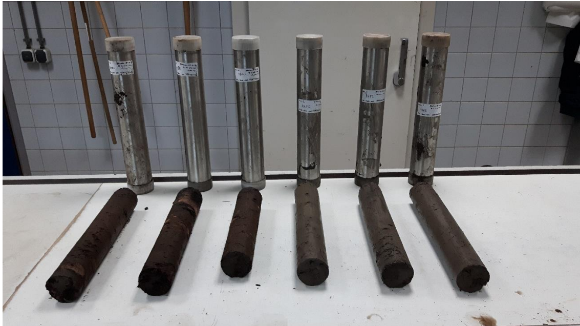
Figure F.1; The undisturbed soil samples extruded from the Ackermann tubes. The contents of tubes 8, 9, 10, 1, 4 and 5 are shown from left to right containing peat (the three most left tubes) and organic clay (the three most right tubes).
