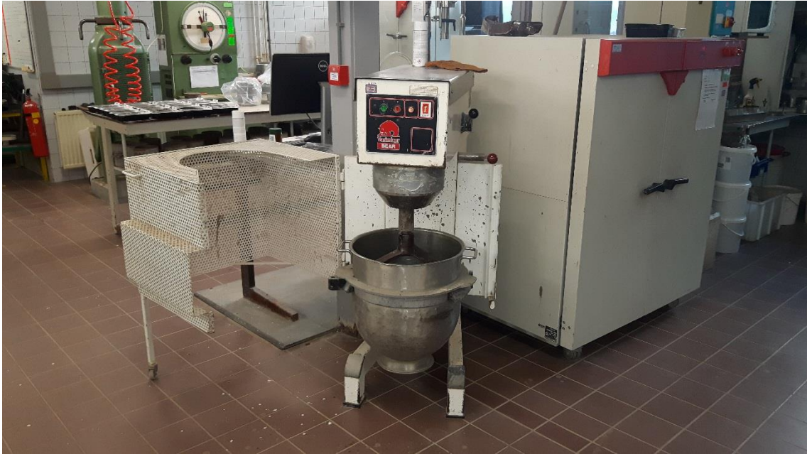
Figure D.3; The Varimixer type 94/AR60 as used in this research for the laboratory soil stabilisation.
