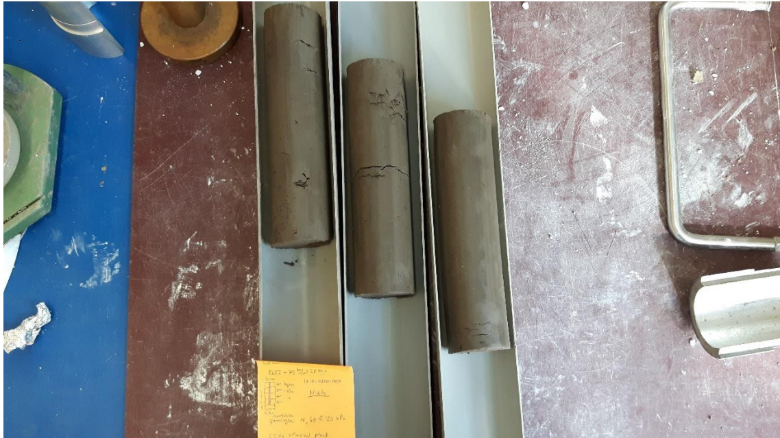
Figure D.11; Extruded stabilised soil samples of 50 mm in diameter.
