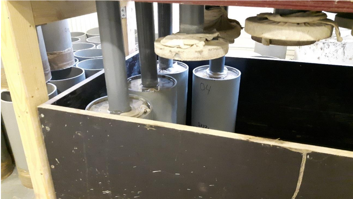
Figure D.7; The container of the mass stabilisation setup filled with a few moulds.
