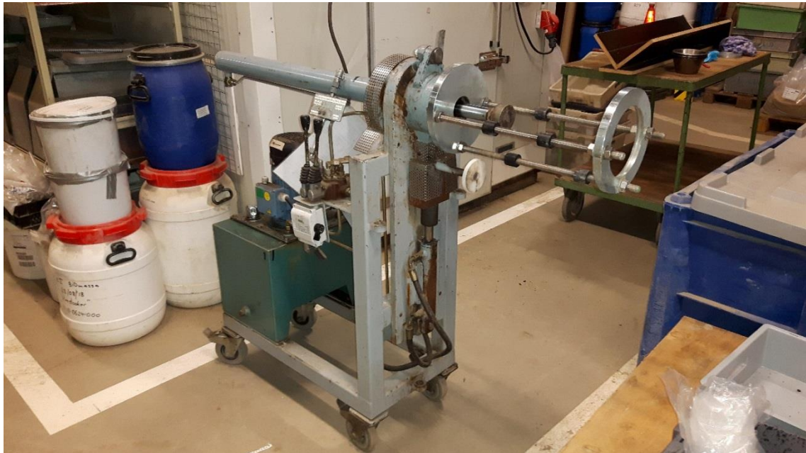
Figure D.9; The extrusion machine that was used to extrude the stabilised soil samples from the moulds.
