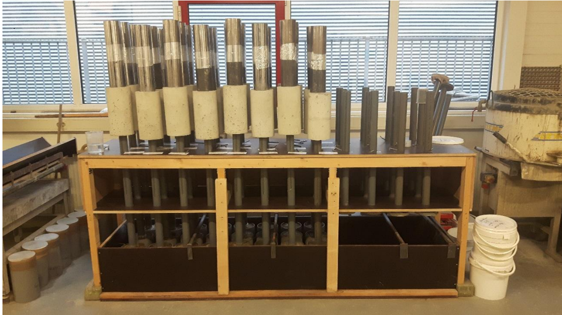
Figure D.1; The mass stabilisation test setup built by Fugro NL Land B.V. used during this research.
