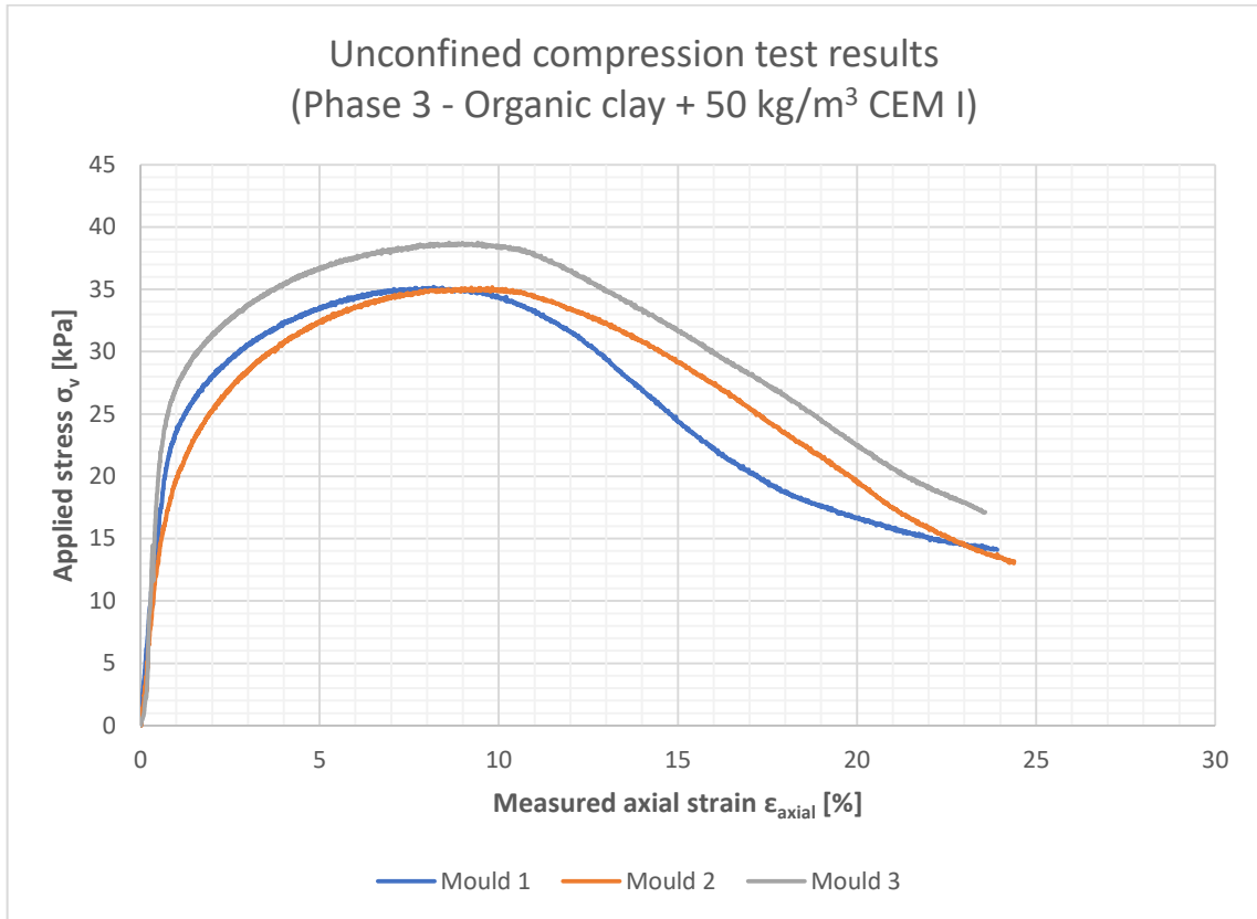
Figure F.62; The stress-strain diagrams obtained from the unconfined compression tests for the organic clay samples stabilised with 50 kg/m 3 of Portland cement (CEM I) in phase 3 of the laboratory research.
