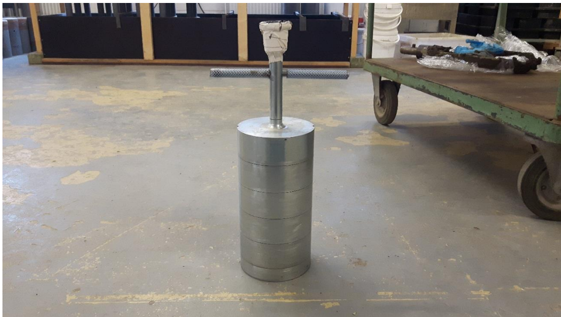
Figure D.5; The metal masher that was used for the compaction of the mixtures in the moulds.
