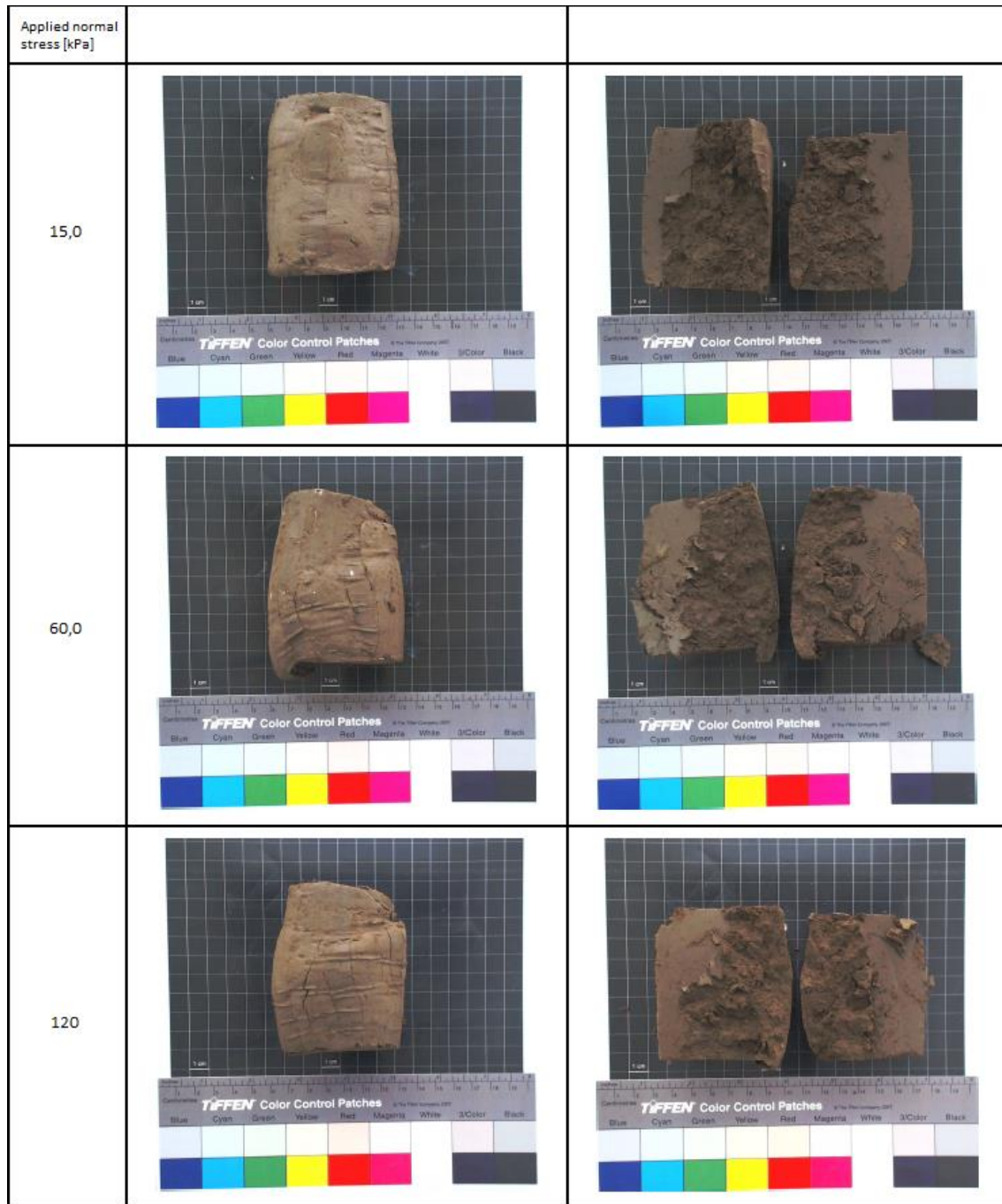
Figure F.104; Photographs of the (undisturbed) stabilised organic clay samples after failure in the isotropically consolidated undrained triaxial test at three different consolidation stresses.
