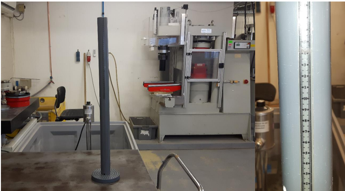
Figure D.8; The plastic mashers that are part of the mass stabilisation setup. These mashers have a measuring tape attached to measure the compression of the mixtures as indicated in the right part of the image.
