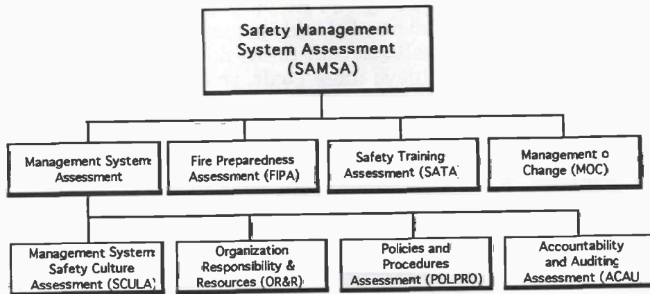
Figure C.12 - Safety Management System assessment module components
