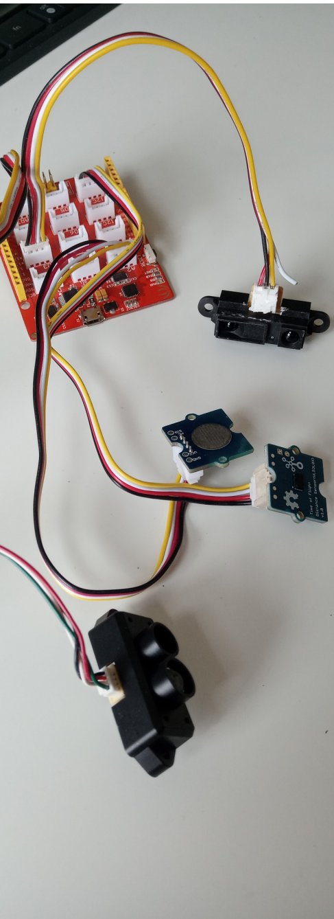
Seeduino with a (from top to bottom) infrared proximity sensor, touch sensor, Time of flight sensor and mini LiDAR sensor
