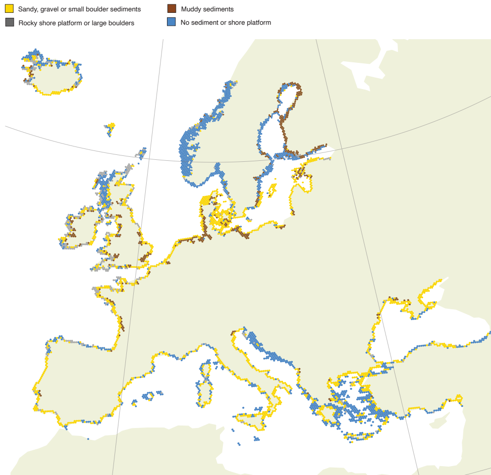
Figure C.3: Map of continental Europe with predicted sediment type , aggregated on a level-5 H3 hexagonal grid for visualization purposes using majority class (mode) per cell. This continental view summarizes around 1.2 million classified coastal transects, highlighting regional patterns. Basemap: Natural Earth.
