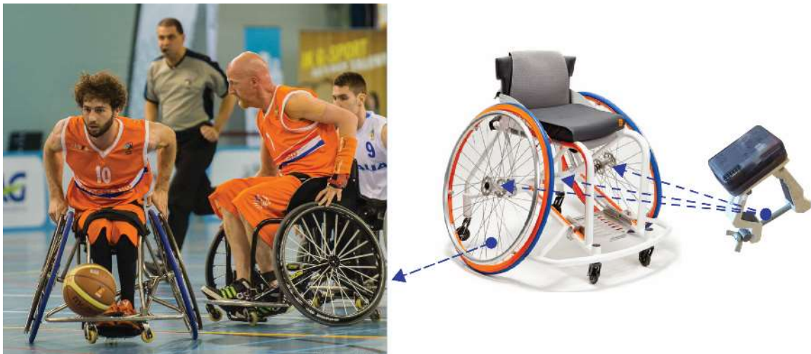
376 Figure 1. Measurement setup, with IMUs on wheels and frame and measurements during a match. (Photograph 377 by www.frankvanhollebeke.be ).
