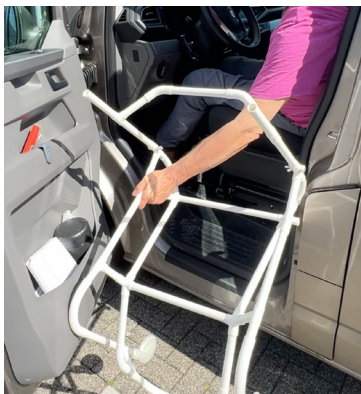
Figure 117. User lifts the frame with the casters still resting on the ground to detach the rear wheels (rear wheels were not prototyped)
