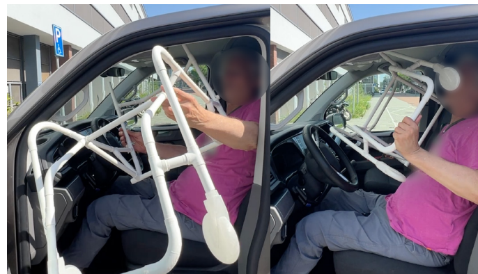
Figure 119. Rotating the frame behind the steering wheel. The casters are pointing towards the open doorframe. Since the fixed backrest extends the frame further, this isn't advisable to do in cars where space is limited.
