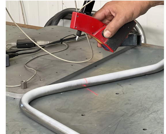
Figure 131. Scanning the seat-to-caster tube | Tube coated in white paint for easier scanner recognition
