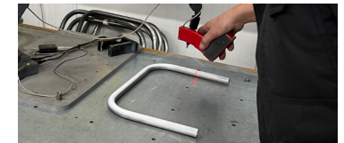
Figure 38. Scanning the tube
