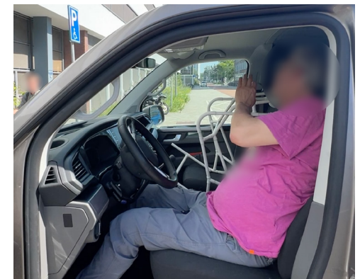
Figure 120. The user places the frame on the passenger seat with the dirty casters facing the seat. Note: in the picture the backrest is slightly tilted upwards because the prototype doesn't have a fixed backrest.
