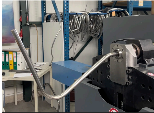
Figure 130. Extrusion of the seat-to-caster tube
