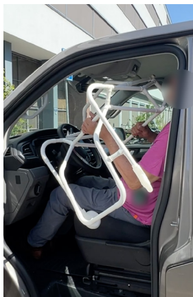
Figure 122. Rotating the frame behind the steering wheel. The casters are pointing towards the open doorframe
