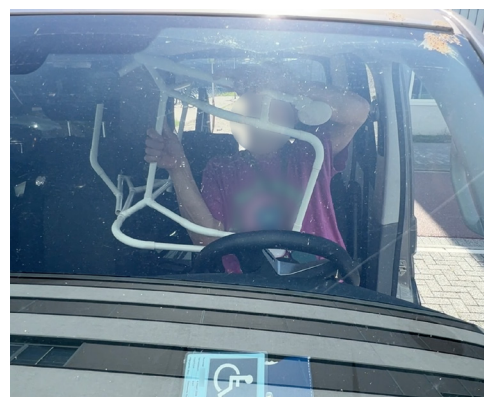
Figure 126. User rotates the frame with the casters pointing outside
