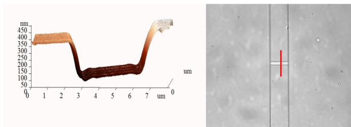
Figure A.1: Left: 3D profile of nanochannel in PDMS captured using AFM. 0 on the y-axis corresponds to the bottom surface of the nanochannel. Right: Channels in PDMS. Red line indicates the position along which depth measurement was performed.
