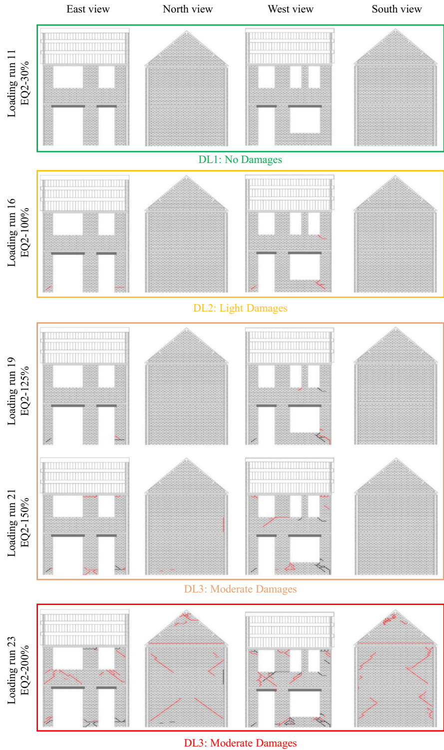
Fig. 12 Damage levels of the EUCENTRE-1 building identified based on its crack propagations [65]
