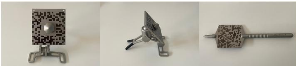
Figure 5: Hardware toolset for AR registration – From left to right: front view of the head device with reference marker, side view of the head device with reference marker, and the pointer.
