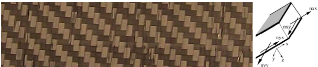
Figure 3: Woven PP sheet, internal membrane forces
