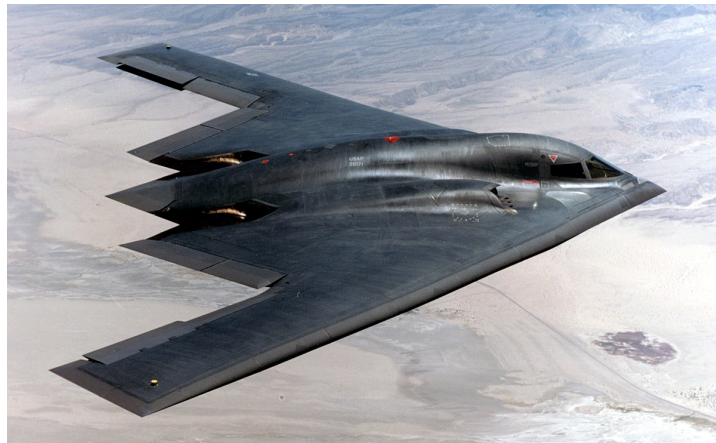
Figure 2.2: B-2 Stealth Bomber employing split rudders for yaw control.
