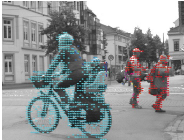
Figure A.5: An estimated optical flow field superimposed on its related frame [10]. .
