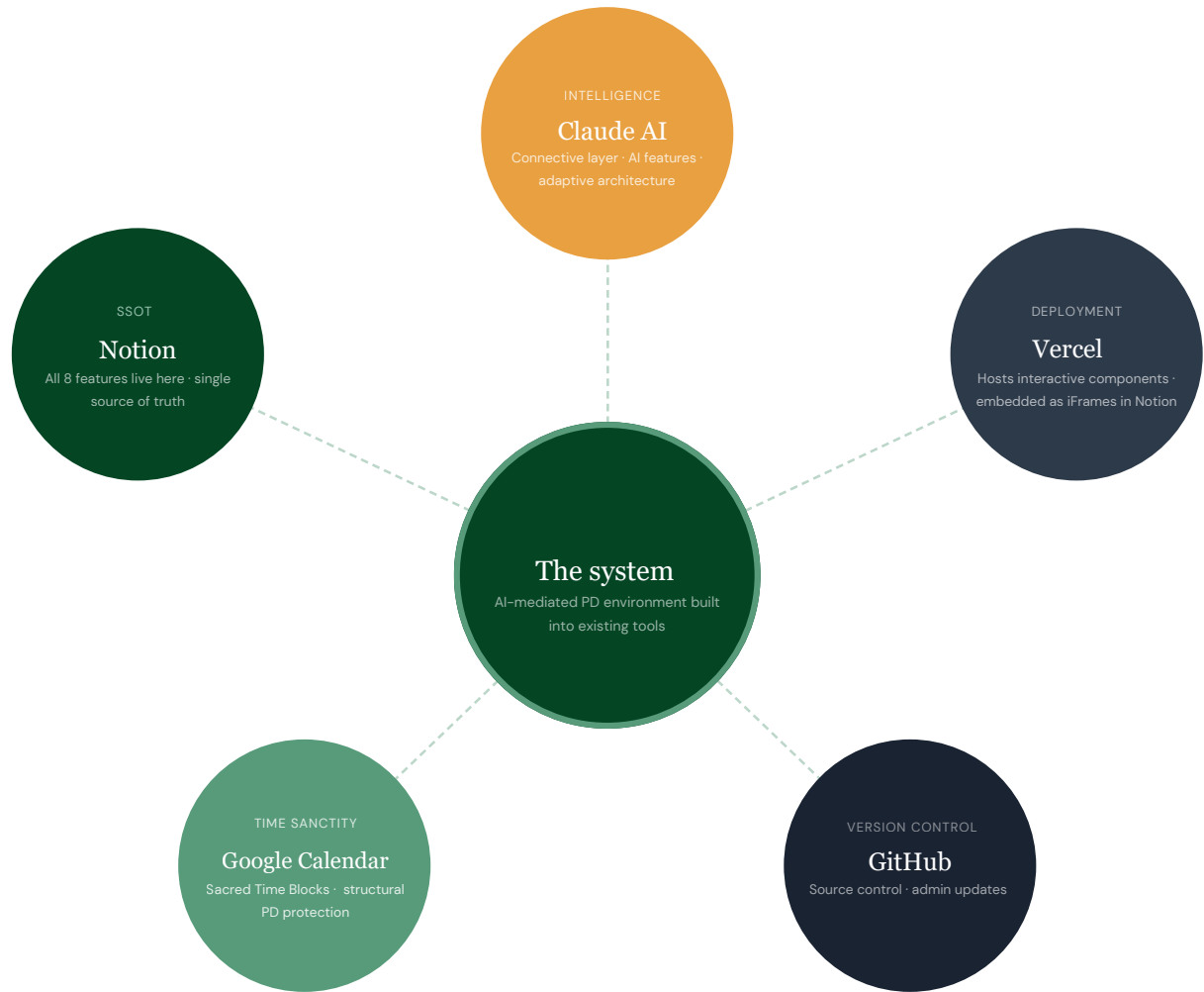
Figure 9 — Platform architecture and ecosystem roles of the made system. The system operates across five interconnected platforms: Notion functions as the single source of truth, housing all features and employee-facing content; Claude AI acts as the connective intelligence layer, linking platforms and enabling adaptive capacity; Google Calendar provides structural time sanctity through programmatic reservation of personal development blocks; Vercel hosts the interactive Claude-built components embedded into Notion as iFrames; and GitHub maintains version control. All five converge in the system — an AI-mediated personal development environment built entirely into the tools Essense already uses.
