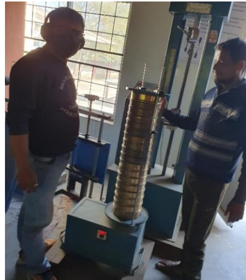
Figure 3: Sieve analysis setup in the lab
