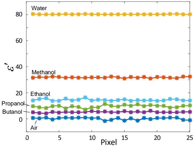
Fig. 5:  $\epsilon'$  of calibration and independent material (ethanol).
