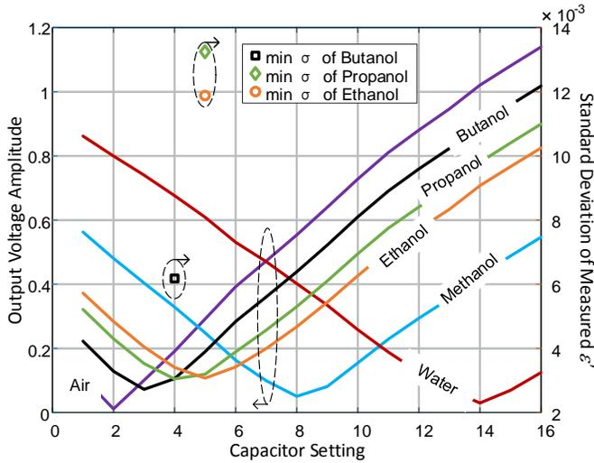
Fig. 4: Normalized output voltage amplitude of center Pixel (pixel 13) versus capacitor setting for 6 materials at 900 MHz, and the corresponding lowest standard deviation ( $\sigma$ ) of chosen independent material.
