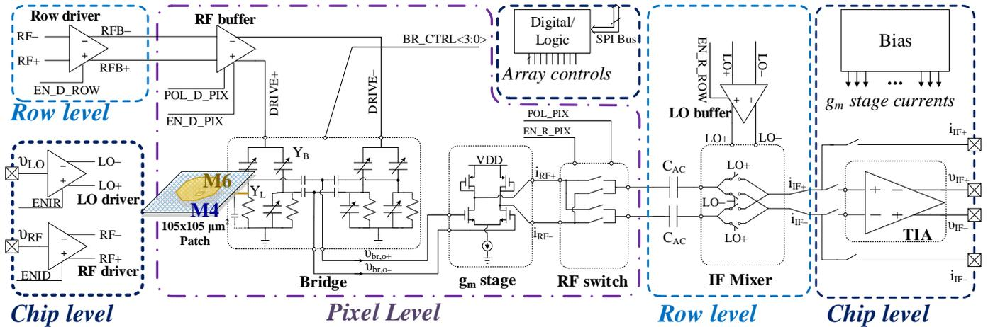
Fig. 2: Sensor matrix readout architecture.
