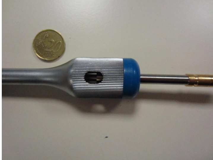
FIGURE 2: In the pictures above we see the Medtronic drill, the CSD department want them to change the design so that the blue cap can be taken off to allow for easier rinsing and brushing furthermore they want to slide the whole rod out so they can rinse and brush through the shaft so change either end of the rod so that is possible. .
