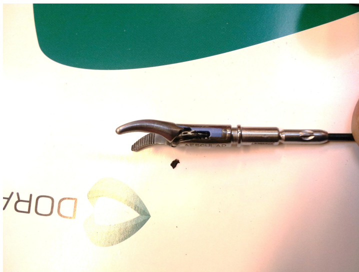
FIGURE 15: 4-bar Aesculap grasper with a crack in the protection layer.
