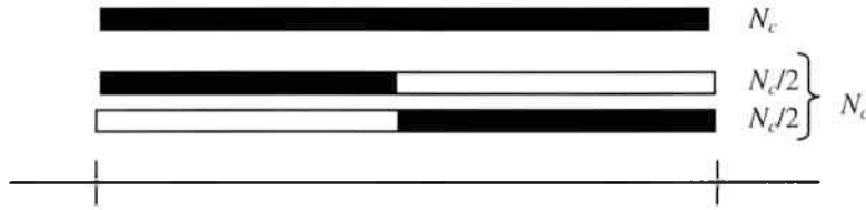
Figure 2.4: Length of the codes in a MPG scheme for one real user with PG equal to the even number of chips N_c and two virtual users belonging to another real user with PG of N_c/2 .
