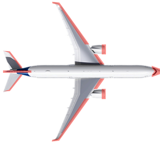
Fig. 2. Bird strike critical zone for the A350-1000, which has a wingspan of 64.75, comparable to the Flying-V.
