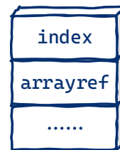
Figure 3.2: Operand Stack When Loading
