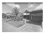
Ave. Size: 200 m²Material: plastered brickworkHeight: 1-2 storeysYear: est. 1970Condition: sufficient
