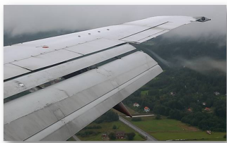
Figure 7.8: Triple slotted flap [28].
