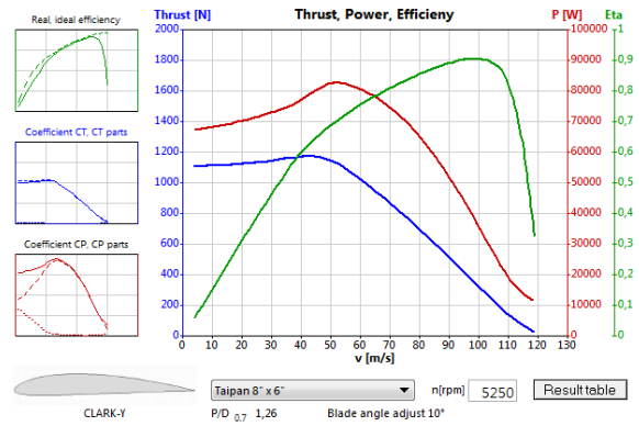
Figure 10.8: Propeller performance at 10° pitch angle
