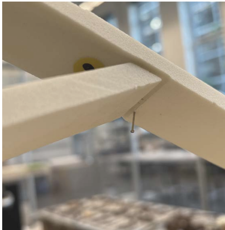
Fig 5.18: Misalignments in prototyping assembly due to the cumulative sum of tolerances with each successive joint. A more robust method of calibration and ensuring higher precision is required.
