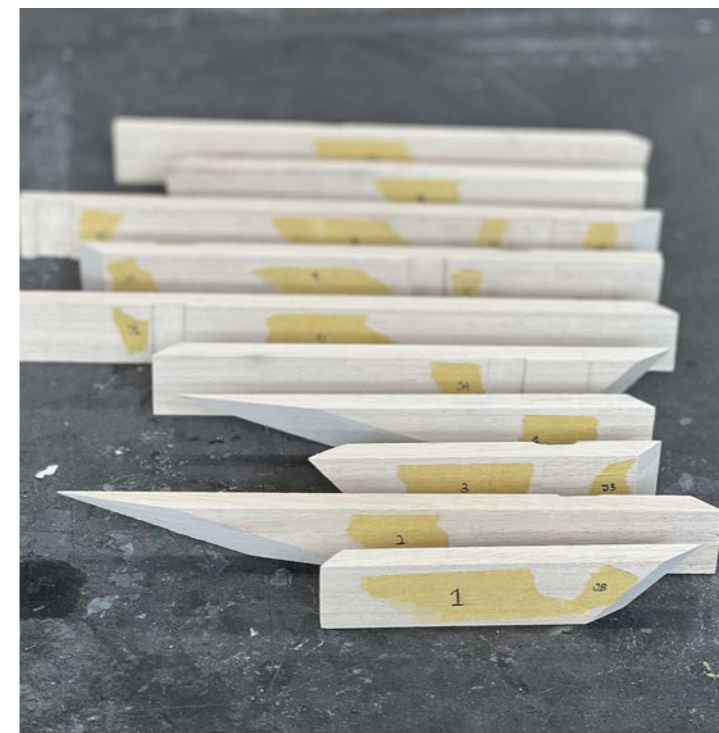
Fig 5.17: Fabrication of Timber and Foam slats with labelling and to allow for more intuitive matching of joint index (yellow sticker) and identification of member index (white sticker)
