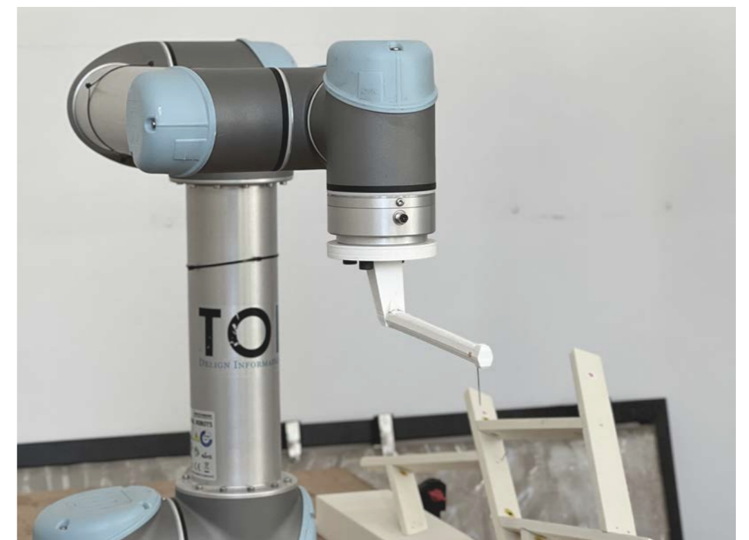
Fig 5.20: New magnetic gripper G6 with a pin attached.
