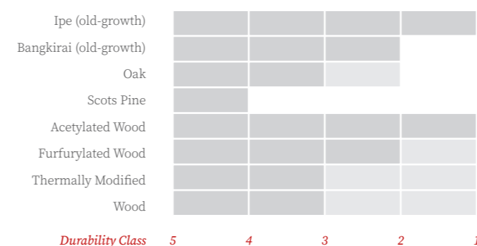
Fig 2.7: Durability comparison (EN 350), adapted from Tomorrow's Timber (Lugt & Harsta, 2020).
