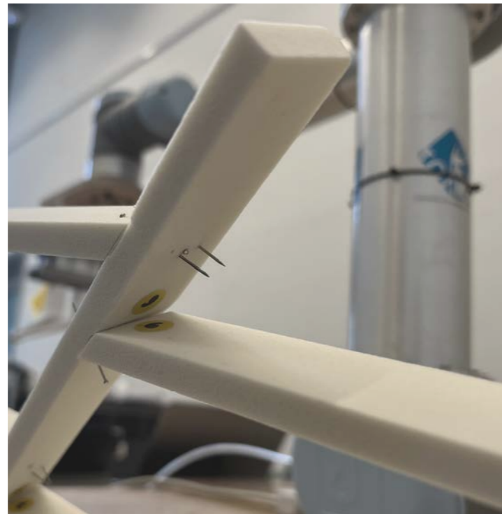
Fig 5.18: Misalignments in prototyping assembly due to the cumulative sum of tolerances with each successive joint. A more robust method of calibration and ensuring higher precision is required.
