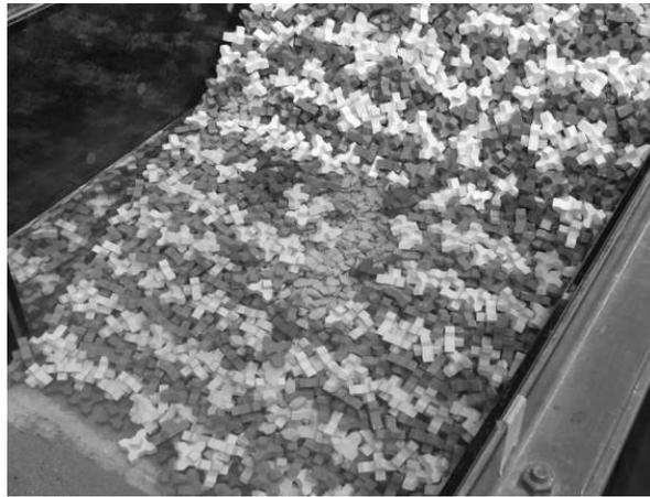
**Figure 3. Failure of the armour layer and exposure of the first underlayer.**
