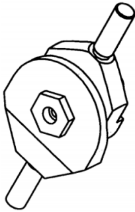
Figure 3.6: Sketch of a deployed self-latching hinge (copy of fig. 2.24) [30]
