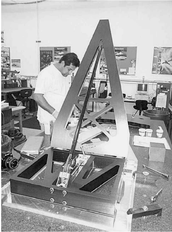
Figure 3.4: Photo of the deployment mechanism of the lidar prototype design [37]
