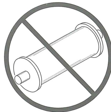
Figure 5.39: Example of a flanged roller. Flanged roller should not be used since they are per definition overconstrained [85]
