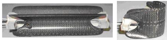
Figure 3.26: A TEMBO CTD-BG1.3 EMC hinge with embedded heater in deployed and stowed configuration [40]
