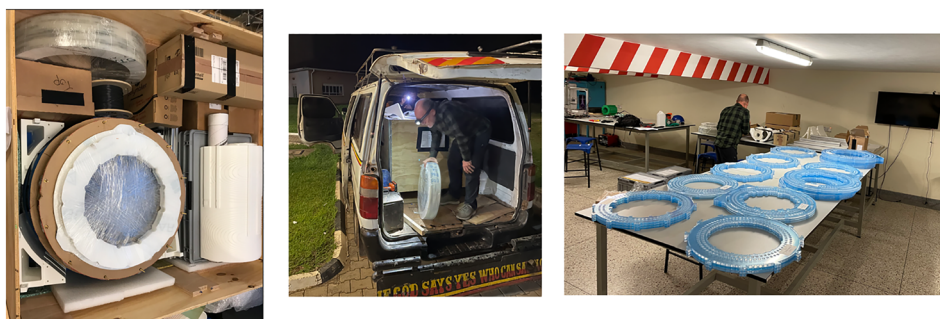
FIGURE 2 Left, Crate containing all components including assembly tools, overall size 1.2 \text{ m} \times 1.0 \text{ m} \times 0.8 \text{ m} and weight 325 kg. Center, Final delivery after two weeks en route, via taxi from the closest airport 5 h away. Right, Illustration of individual plastic rings for the magnet.
