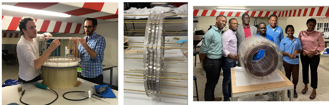
FIGURE 5 Magnet assembly. Left, Brass rods are used to align each of the rings of the magnets. Nuts are used as spacers between each ring. The forces between the rings are significant but not dangerous. Center, After each ring is threaded onto the rods, the position of each nut is carefully adjusted so that there is equal spacing between each of the rings, and they are precisely aligned parallel to each other. Right, The completed magnet consisting of 25 rings, the central 17 containing two layers of magnets, and the front/back three rings having three layers.
