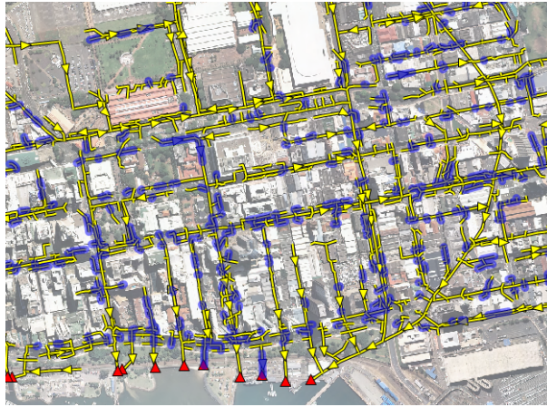
Figure H.9: Blocked conduits (blue colour)
