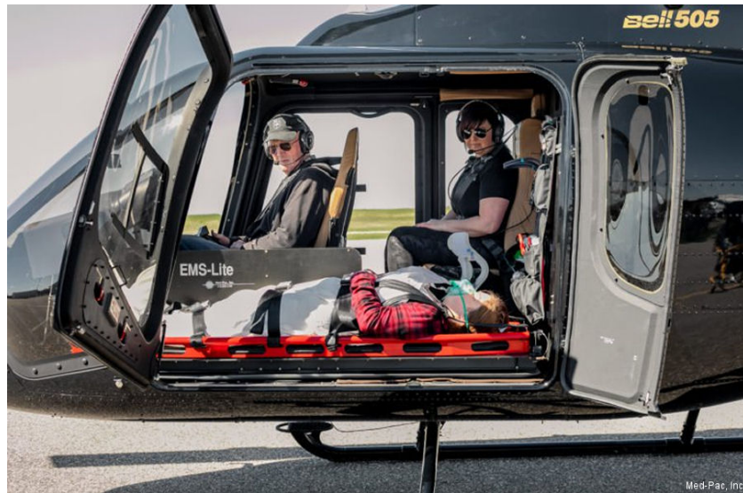
Figure 6.1: Fuselage layout displaying the seating arrangement for pilot, medical personnel, and passenger [43]
