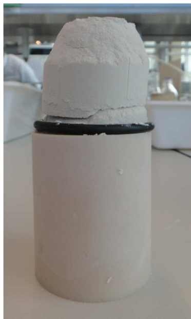
Figure III - 5: Core and external filter cake ( 39 \pm 0.5 mm) of experiment 1C; the filter cake is very brittle. By removing the core and external filter cake from the core holder the top of the external filter cake crumbled. At the bottom a crack is visible; this is caused by the removal from the core holder. The black ring is one of the O-rings used to seal the set-up.
