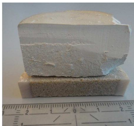
Figure 11: Top part of the core of experiment 1A, used for ESEM characterisation and external filter cake ( 20 \pm 0.5 mm)
