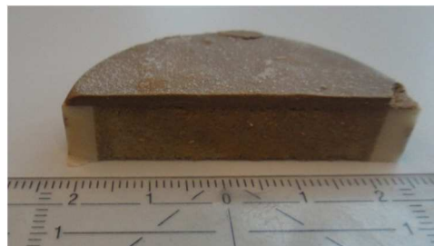
Figure III - 14: Top part of the core of experiment 4 and external filter cake ( 1.92 \pm 0.05 mm)
