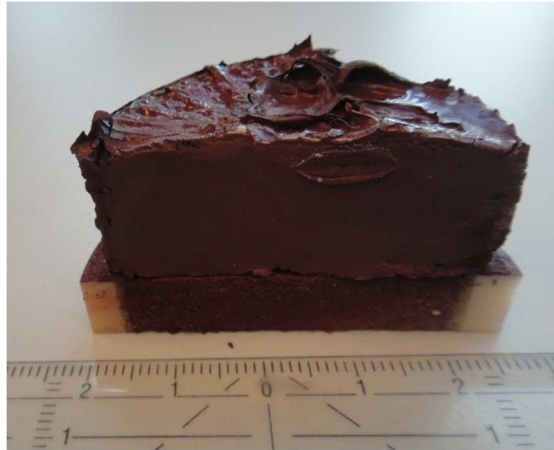
Figure 29: Top part of the core and external filter cake ( 17 \pm 0.5 mm)
