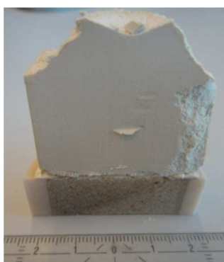
Figure 17: Top part of the core of experiment 2A, external filter cake is 35 \pm 0.5 mm
