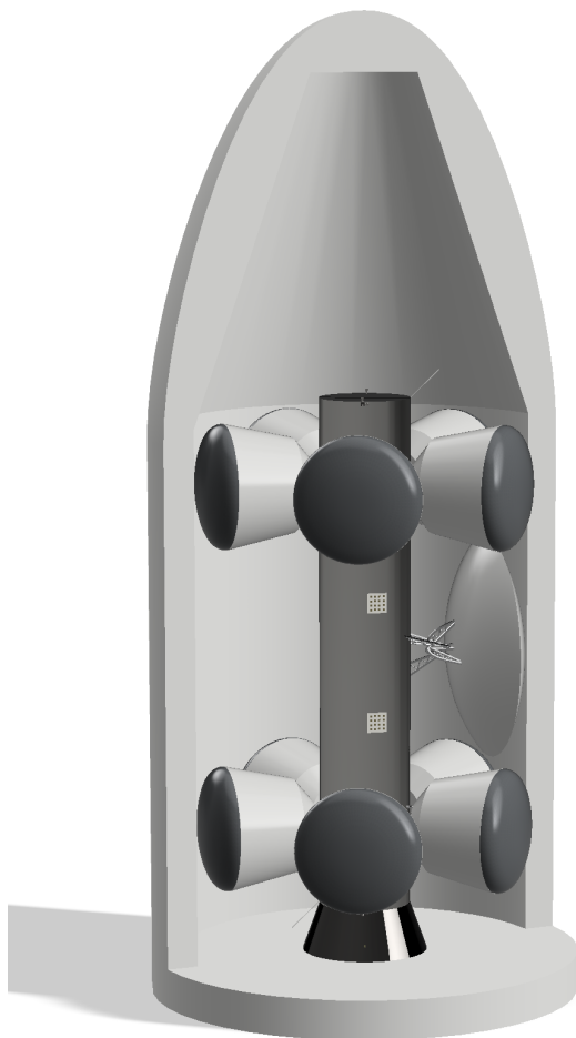
Figure 9.1: The orbiter's configuration at launch
