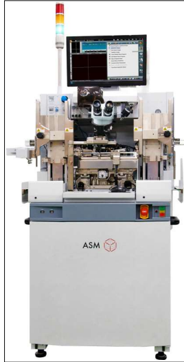
Fig. 6. Commercial wirebonder from ASMPT consisting of an xyz -stage
