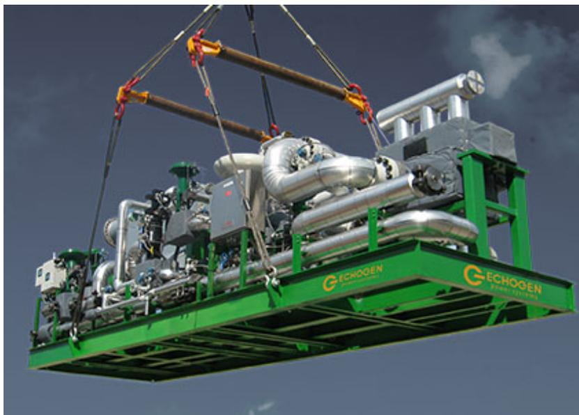
Figure 7.5: Echogen's 8 MW CO<sub>2</sub> RC-based waste heat recovery module EPS100 [28].
