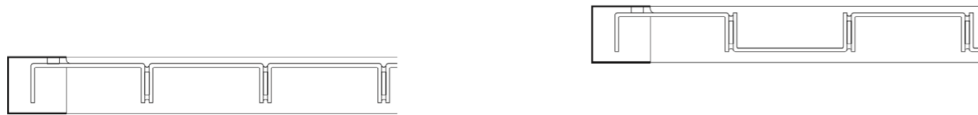
Figure 20 and 21. Single leaf profiled glass installation From “Glass Construction Manual” (2nd ed., p 63), by Schittich, Staib, Balkow, Schuler, & Sobek. (2007).
