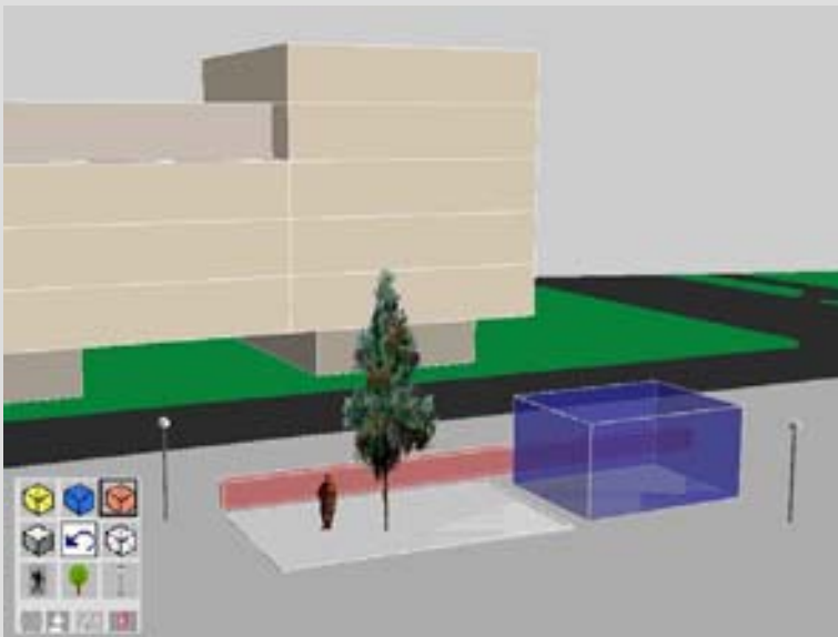
Figure 66. Sketch with some elementary objects and semi transparent volumes, seen in relation to a building with and without façade textures and from different points of view.
