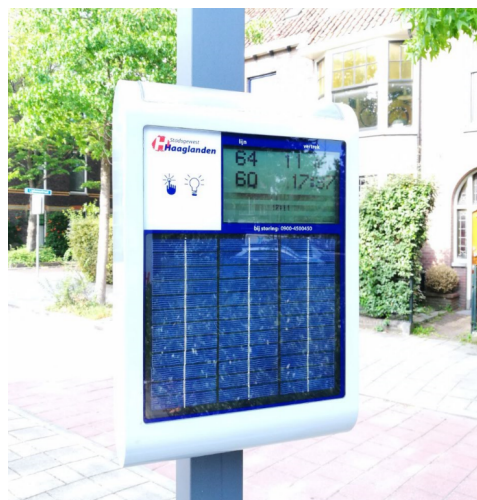
Figure 1.5: Solar-powered LCD for indicating the time to the next bus or tram
