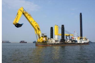
Figure 1. Offshore excavator
